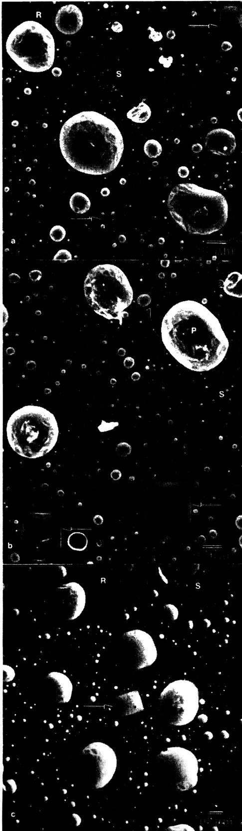
FIG. 1. (a)–(c) SEM micrographs of an InP(001) surface after thermal treatment at 500°C for 10 min in ultrahigh vacuum. Morphologies and symbols are discussed in the text.
