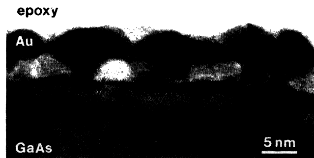
FIG. 2. Cross-sectional transmission electron microscopy image of a Au/oxide/GaAs(100) diode prepared by ion milling at low temperatures. The top layer with lattice fringes visible is polycrystalline Au and the phase closer to the interface is the oxide. The darker layer with fringes right at the interface is perhaps an indication of a reaction beginning with the substrate (300 keV, [110] pole).
