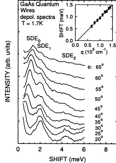
FIG. 4. Depolarized light scattering spectra of the quantum wire sample for different tilt angles  $\Theta$ , corresponding to different wave vectors  $q$  along the wires. The inset shows the wave-vector dispersion of the intrasubband spin-density excitation ( $SDE_0$ ).
