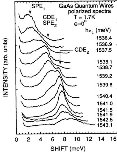
FIG. 3. Polarized resonant light scattering spectra of 1D intersubband excitations for different incident photon energies.
