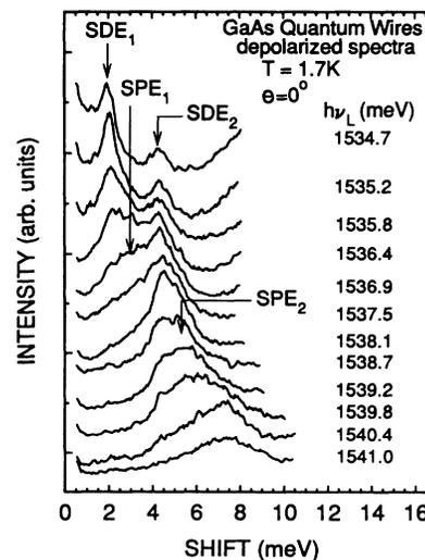
FIG. 2. Depolarized resonant light scattering spectra of 1D intersubband excitations for different incident photon energies.
