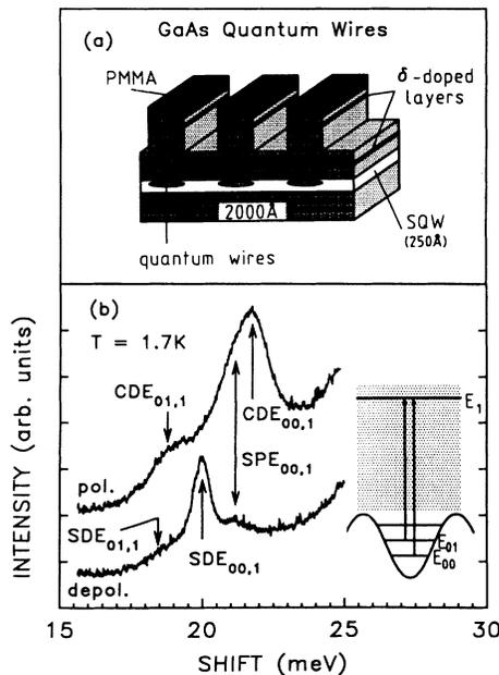
FIG. 1. (a) Schematic structure of the quantum wires. The lateral carrier confinement is achieved by shallow dry etching through the openings of the PMMA resist mask. (b) Polarized and depolarized light scattering spectra corresponding to 2D-like transitions to the first excited subband due to the confinement in the growth direction, as shown in the inset.
