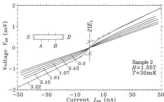
FIG. 1. Typical nonlinear current-voltage dependencies, taken with four-probe dc technique in the vicinity of the critical point, in the ES phase. Dashed lines and arrows explain the procedure used to extract  $E_t$  from the  $I$ - $V$  curves. The inset shows the sample top view.  $S$  and  $D$  are the current probes,  $A$ ,  $B$  are potential probes. The  $\delta n_s = n_c - n_s$  value for each  $I$ - $V$  curve is shown in units of  $10^9$  cm<sup>-2</sup>.
