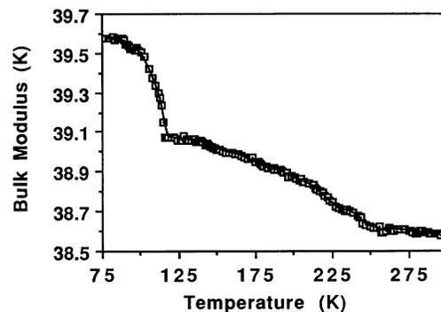
FIG. 7. Bulk modulus of high- $T_c$  superconductor  $\text{GdBa}_2\text{Cu}_3\text{O}_{7-\delta}$  as a function of temperature.
