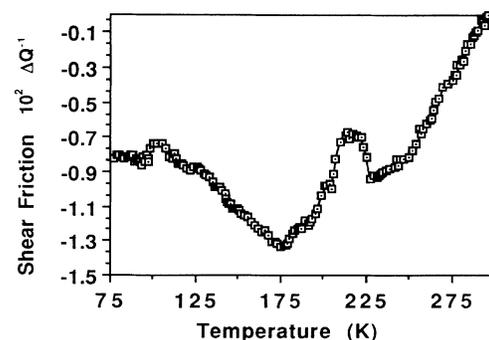
FIG. 11. Temperature dependence of shear internal friction for high- $T_c$  superconductor  $\text{GdBa}_2\text{Cu}_3\text{O}_{7-\delta}$ .
