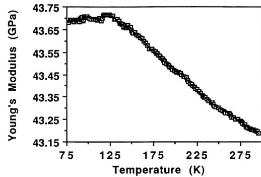
FIG. 5. Young's modulus of high- $T_c$  superconductor  $\text{GdBa}_2\text{Cu}_3\text{O}_{7-\delta}$  as a function of temperature.
