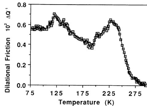
FIG. 10. Temperature dependence of dilational internal friction for high- $T_c$  superconductor  $\text{GdBa}_2\text{Cu}_3\text{O}_{7-\delta}$ .
