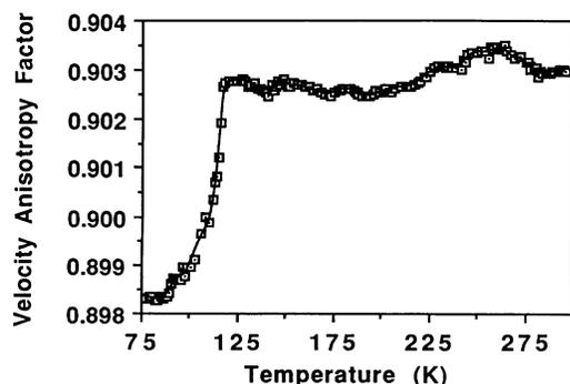
FIG. 4. Acoustic wave velocity anisotropy factor vs temperature in high- $T_c$  superconductor  $\text{GdBa}_2\text{Cu}_3\text{O}_{7-\delta}$ .
