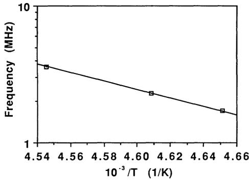
FIG. 12. Arrhenius plot of ultrasonic frequency for low-temperature peak in high- $T_c$  superconductor  $\text{GdBa}_2\text{Cu}_3\text{O}_{7-\delta}$ .
