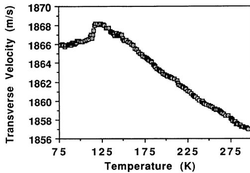
FIG. 3. Transverse wave velocity vs temperature at high- $T_c$  superconductor  $\text{GdBa}_2\text{Cu}_3\text{O}_{7-\delta}$ .
