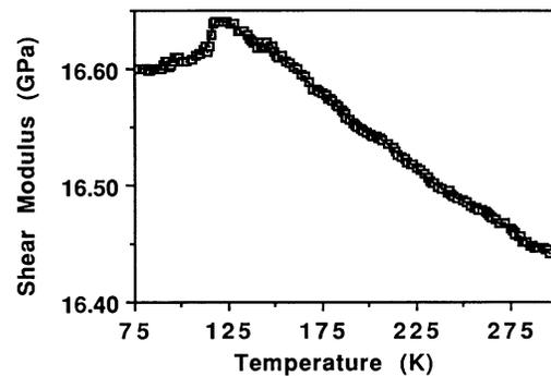
FIG. 6. Shear modulus of high- $T_c$  superconductor  $\text{GdBa}_2\text{Cu}_3\text{O}_{7-\delta}$  as a function of temperature.
