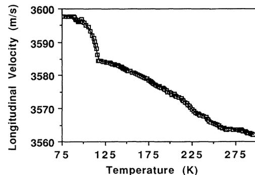
FIG. 2. Longitudinal wave velocity vs temperature at high- $T_c$  superconductor GdBa<sub>2</sub>Cu<sub>3</sub>O<sub>7- $\delta$</sub> .
