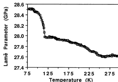
FIG. 8. Lamé parameter of high- $T_c$  superconductor  $\text{GdBa}_2\text{Cu}_3\text{O}_{7-\delta}$  as a function of temperature.
