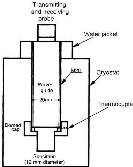
FIG. 1. Design of short-specimen buffer-rod system. The 20-mm-long specimen is mechanically coupled to 50-mm-long buffer rod. Cupler is of stainless steel SUS 304 (U.S. designation; SAE 30304).
