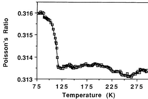
FIG. 9. Poisson's ratio of high- $T_c$  superconductor  $\text{GdBa}_2\text{Cu}_3\text{O}_{7-\delta}$  as a function of temperature.
