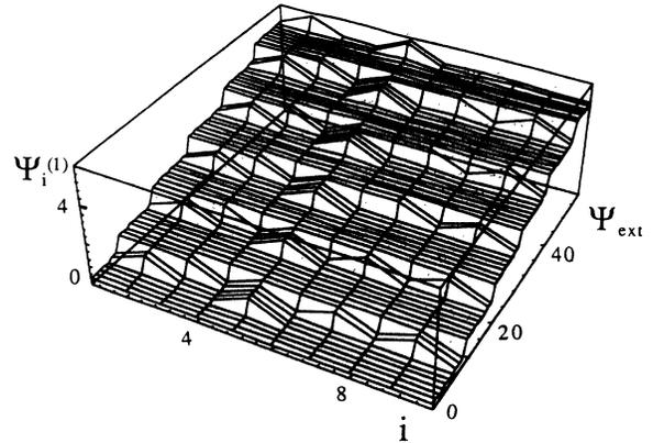
FIG. 2. Normalized flux  $\Psi_i^{(1)}$  in the external row of intergranular loops of area  $S_0$  versus the normalized applied flux  $\Psi_{\text{ext}}$ . The  $i$  label represents the angular position of the elementary intergranular loops. The system has been assumed to be completely uniform [ $\alpha_{ki} = 1$  for any pair  $(k,i)$ ] and immersed in a finite-temperature bath.
