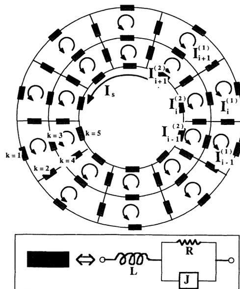
FIG. 1. Simplified 2D network of Josephson junctions and inductances. One rectangle contains an inductance  $L$  and a JJ, schematized through the RSJ model, as shown in the inset. The currents  $I_i^{(j)}$  circulating in each intergranular loop of area  $S_0$  and the inner loop current  $I_s$  are also shown.
