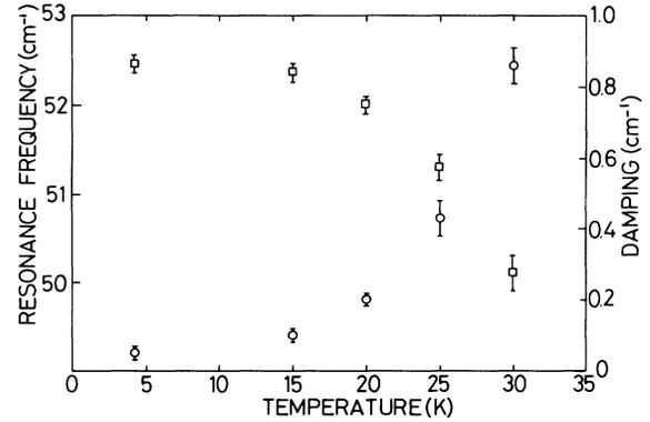
FIG. 2. Temperature dependence of the resonance frequency ( $\square$ , left-hand axis) and damping ( $\circ$ , right-hand axis) determined by a fit of theory to the data of Fig. 1.
