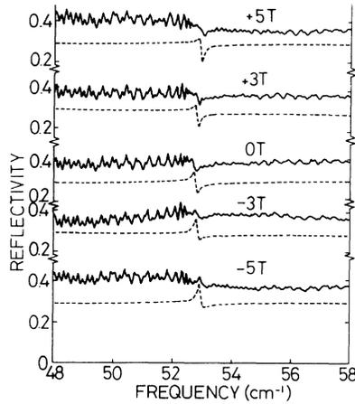
FIG. 4. Spectra at various fields in  $s$  polarization for the crystal  $c$  axis transverse to the magnetic field, i.e., horizontal. — experiment, - - - theory. Resolution:  $0.063 \text{ cm}^{-1}$ , fitting parameters as for Fig. 3.
