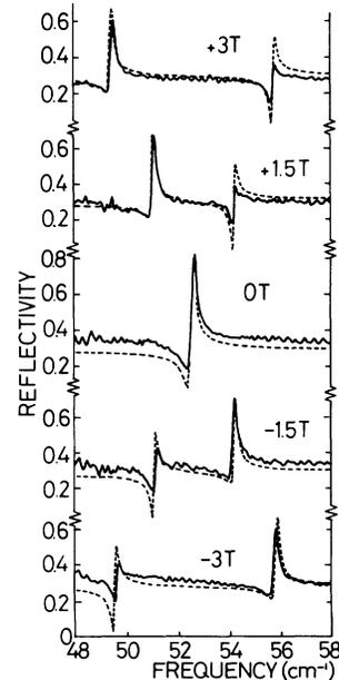
FIG. 3. Magnetic-field splitting of the 4.2-K spectrum in the geometry of Fig. 1. — experiment, - - - theory. Resolution:  $0.125 \text{ cm}^{-1}$ . The theoretical curves were drawn with  $\epsilon = 5.5$ ,  $\omega_r = 52.45 \text{ cm}^{-1}$ , as determined from the 0-T spectrum, and  $\Gamma = 0.05 \text{ cm}^{-1}$ .
