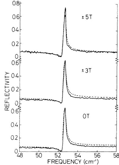
FIG. 5. Spectra at various fields in  $p$  polarization for the crystal  $c$  axis horizontal. — experiment, - - - theory. Resolution:  $0.063 \text{ cm}^{-1}$ , fitting parameters as for Fig. 3.
