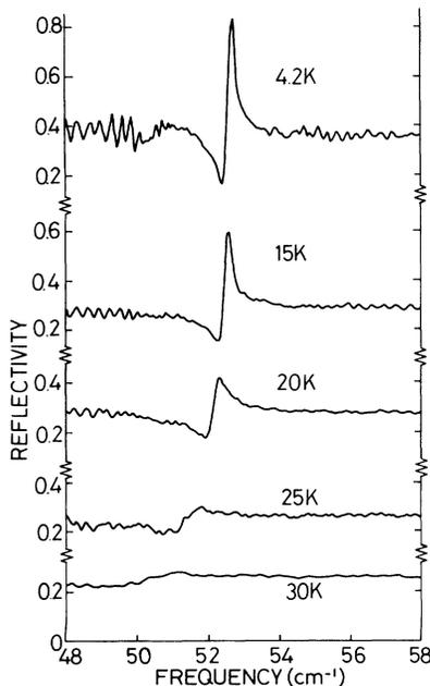
FIG. 1. Frequency scans of  $45^\circ$  reflectivity in  $s$  polarization through magnetic resonance in zero field for a range of temperatures. The crystal  $c$  axis is along the magnetic field, i.e., vertical. Resolution:  $0.25 \text{ cm}^{-1}$  at 30 K,  $0.125 \text{ cm}^{-1}$  at other temperatures.
