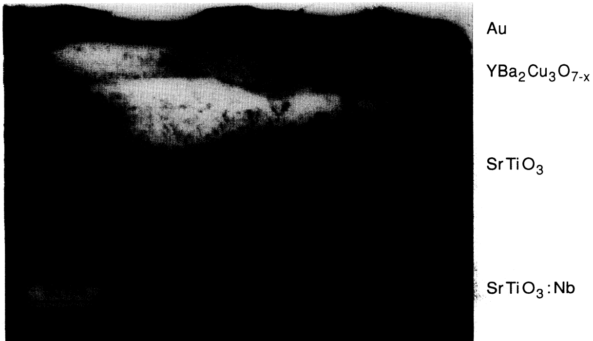
FIG. 9. TEM micrograph of an Au/YBa 2 Cu 3 O 7-x /SrTiO 3 /SrTiO 3 :Nb heterostructure. This bright field image shows dislocations seen as shades and dark traces coming to the surface of the SrTiO 3 :Nb substrate in addition to the homoepitaxial SrTiO 3 layer with a higher dislocation density and a rather rough upper surface. Interestingly the YBa 2 Cu 3 O 7-x upper surface is somewhat flatter. Also visible in this image is the top electrode of polycrystalline gold. Arrows indicate the SrTiO 3 /SrTiO 3 :Nb interface.
