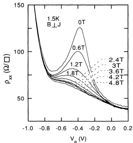
FIG. 4. The transverse magnetic field  $B\perp$  dependence of  $\rho_{xx}$  plotted as functions of  $V_g$ .
