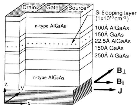
FIG. 1. The cross-sectional view of the sample structure is schematically shown. The channel is taken in the  $x$  direction. An in-plane magnetic field is applied both in the  $x$  and  $y$  direction.
