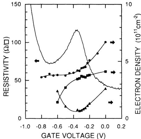
FIG. 2. The zero-field channel resistivity  $\rho_{xx}$ ; gate voltage  $V_g$  characteristic at 1.5 K is shown by a solid line. Closed circles and squares indicate the electron densities of individual subbands. Closed triangles are the difference between them.
