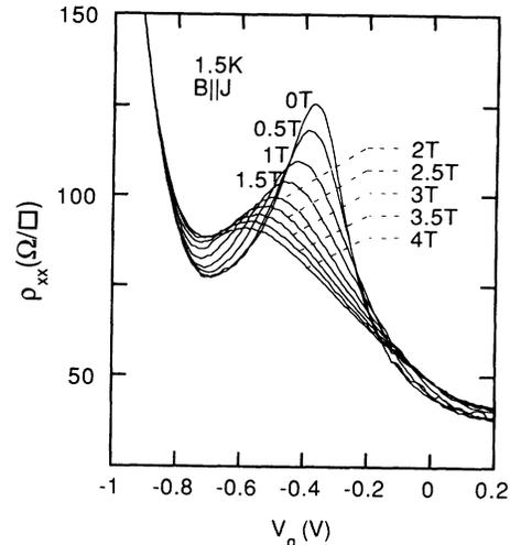
FIG. 3. The longitudinal magnetic field  $B\parallel$  dependence of  $\rho_{xx}$  plotted as functions of  $V_g$ .
