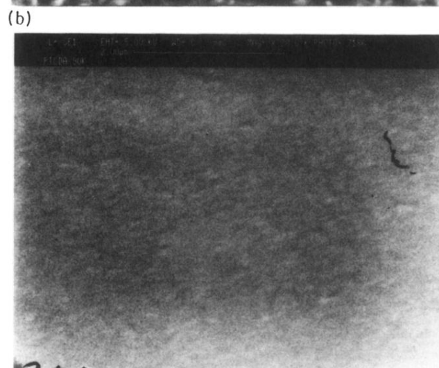
FIG. 7. Scanning electron microscope images of the surface of a PTCDA film grown on glass at a substrate temperature of (a) 293 and (b) 90 K.
