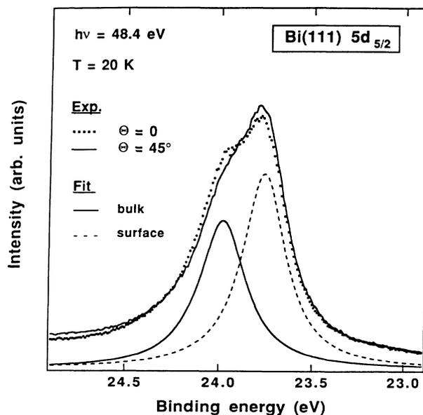
FIG. 5. Bi  $5d_{5/2}$  core-level spectrum excited with 48.4 eV photon energy at a sample temperature of 20 K. The two Lorentzians resulting from the line-shape analysis (see text) indicate the bulk (full curve) and surface components (dashed curve).
