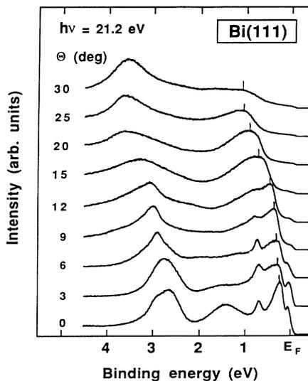
FIG. 3. Off-normal emission spectra of Bi(111) for photon energy of 21.2 eV in the  $\bar{\Gamma}\bar{K}$  direction of the surface Brillouin zone.
