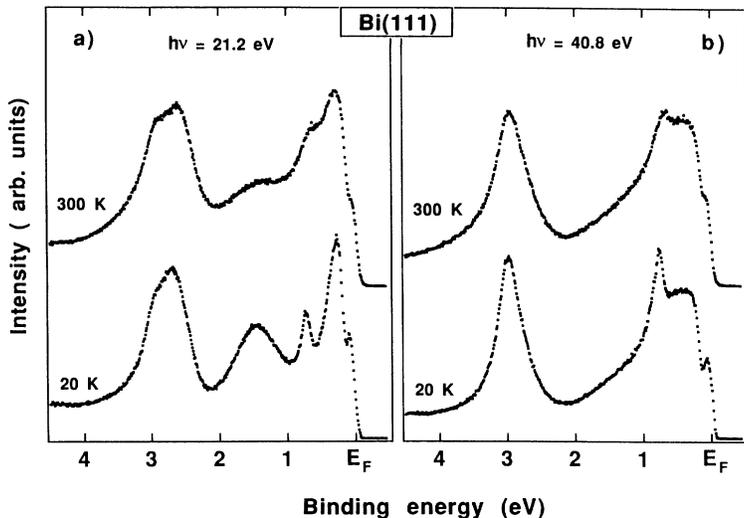
FIG. 1. Photoemission spectra at normal emission from Bi(111) at  $T=300$  K and  $T=20$  K excited with photon energies of (a) 21.2 eV and (b) 40.8 eV.
