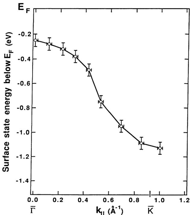
FIG. 4. Dispersion of the surface state energy along the  $\bar{\Gamma}\bar{K}$  direction. The curve connecting the experimental points is drawn to guide the eyes.
