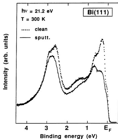
FIG. 2. Influence of surface roughness on the He I (21.2 eV) spectra. The clean Bi(111) surface was sputtered with Ar ions (1 kV, 10  $\mu$ A) and measured at room temperature.
