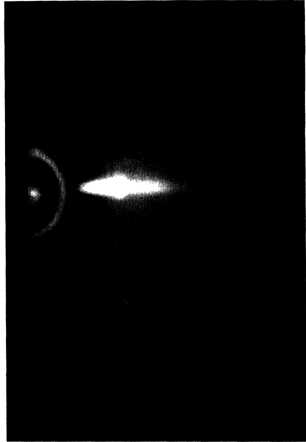
FIG. 7. RHEED pattern taken along the [\bar{2}33] azimuth from the \text{Sb}_4 -stabilized (311) GaAs surface.
