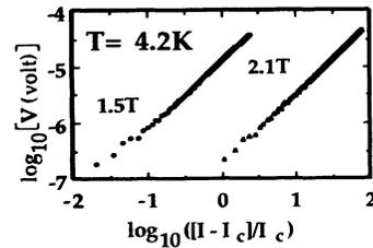
FIG. 4. Typical scaling plots for the  $I$ - $V$  curves at fields below the peak regime ( $H=1.5$  T) and above the peak regime ( $H=2.1$  T) at  $T=4.2$  K. For clarity, the latter data set is shifted up by one and a half decade in the reduced current.
