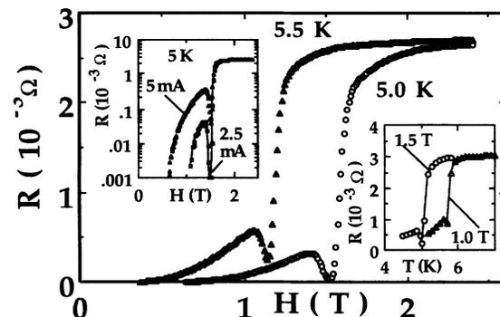
FIG. 1. Peak effect in  $2H\text{-NbSe}_2$  for  $H$  perpendicular to the layers. The minimum in the resistance occurs slightly below  $H$  at both temperatures. The upper inset shows the nonlinearity of the effect through the strong current dependence of the resistance. The lower inset shows the same effect obtained at a fixed field and varying temperature.
