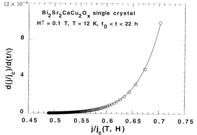
FIG. 2.  $d(j/j_c)/d(t/\tau)$  vs  $j/j_c$  for a single crystal of Bi 2:2:1:2 at  $T = 12$  K. The solid line is the fit to Eq. (7).
