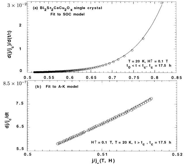
FIG. 3. (a)  $d(j/j_c)/d(t/\tau)$  vs  $j/j_c$  for a single crystal of Bi 2:2:1:2 at  $T = 20$  K, where the solid line is the fit to Eq. (7). (b)  $d(j/j_c)/dt$  vs  $j/j_c$  for a single crystal of Bi 2:2:1:2 at  $T = 20$  K for  $t > t_c$ , where  $t_c$  is the crossover time and the solid line is the fit to the Anderson-Kim model.
