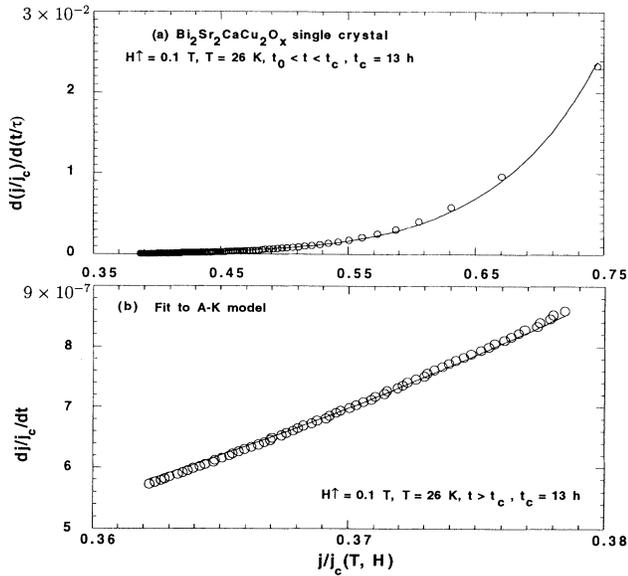
FIG. 4. (a)  $d(j/j_c)/d(t/\tau)$  vs  $j/j_c$  for a single crystal of Bi 2:2:1:2 at  $T=26$  K, where the solid line is the fit to Eq. (7). (b)  $d(j/j_c)/dt$  vs  $j/j_c$  for a single crystal of Bi 2:2:1:2 at  $T=26$  K for  $t > t_c$ , where the solid line is fit to the Anderson-Kim model.
