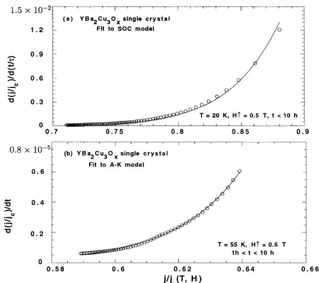
FIG. 9. (a)  $d(j/j_c)/d(t/\tau)$  vs  $j/j_c$  for a single crystal of Y 1:2:3 at  $T = 20$  K, where the solid line is fit to Eq. (7). (b)  $d(j/j_c)/dt$  vs  $j/j_c$  for a single crystal of Y 1:2:3 at  $T = 55$  K for  $t > t_c$ , where the solid line is the fit to the Anderson-Kim model.
