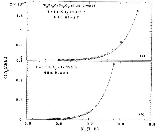
FIG. 6. (a)  $d(j/j_c)/d(t/\tau)$  vs  $j/j_c$  for a single crystal of Bi 2:2:1:2 at  $T=5.5$  K for decreasing field  $H\downarrow=2$  T. (b)  $d(j/j_c)/dt$  vs  $j/j_c$  for a single crystal of Bi 2:2:1:2 at  $T=5.5$  K for increasing field  $H\uparrow=2$  T, where the solid line is the fit to Eq. (7).
