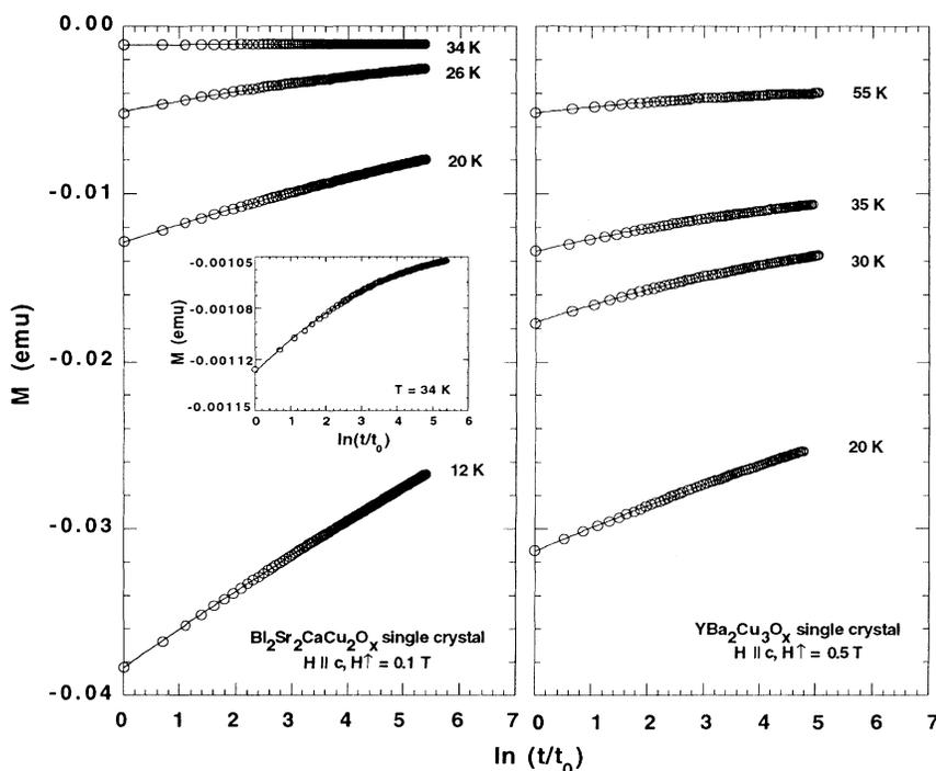
FIG. 1. Magnetization vs  $\ln(t/t_0)$  at 0.1 T applied parallel to the  $c$  axis of single crystals of  $\text{Bi}_2\text{Sr}_2\text{CaCu}_2\text{O}_x$  and  $\text{YBa}_2\text{Cu}_3\text{O}_x$  at temperatures indicated. The solid lines are the fits with  $\ln(t/t_0) + b \ln^2(t/t_0)$  indicating nonlogarithmic relaxation. The inset shows the pronounced nonlogarithmic behavior for Bi 2:2:1:2 at 34 K.
