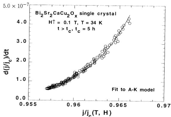
FIG. 5.  $d(j/j_c)/dt$  vs  $j/j_c$  for a single crystal of Bi 2:2:1:2 at  $T=34$  K for  $t > t_c$ , where the solid line is fit to the Anderson-Kim model.
