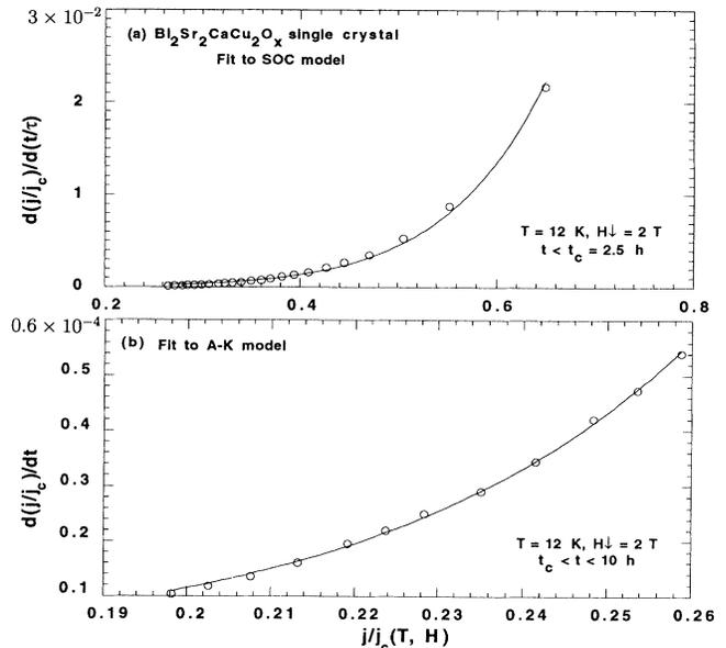
FIG. 7. (a)  $d(j/j_c)/d(t/\tau)$  vs  $j/j_c$  for a single crystal of Bi 2:2:1:2 at  $T=12$  K for decreasing field  $H\downarrow=2$  T, where the solid line is the fit to Eq. (7). (b)  $d(j/j_c)/dt$  vs  $j/j_c$  for a single crystal of Bi 2:2:1:2 at  $T=12$  K for  $t > t_c$ , where the solid line is the fit to the Anderson-Kim model.
