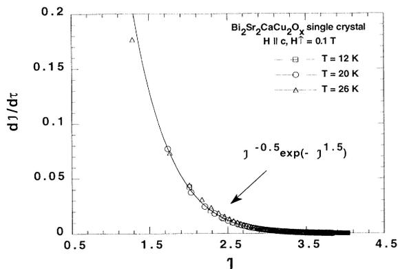
FIG. 8. The universal behavior of the flux-creep rate for a single crystal of Bi 2:2:1:2 normalized by temperature, where the scaled curve is fitted with  $J^{-(\beta-1)} \exp(-J^\beta)$ .
