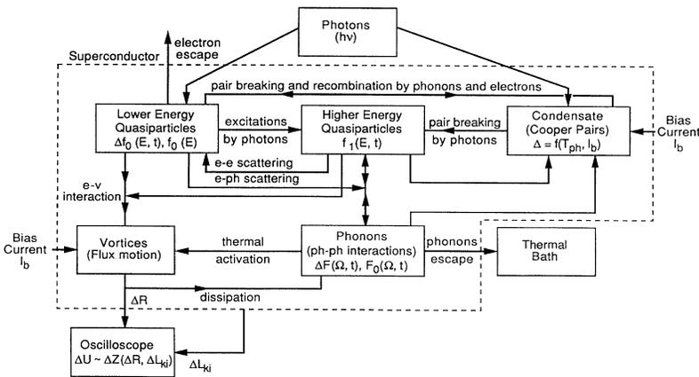
FIG. 2. Block diagram of a superconductor for a nonequilibrium condition created by the optical pulse.
