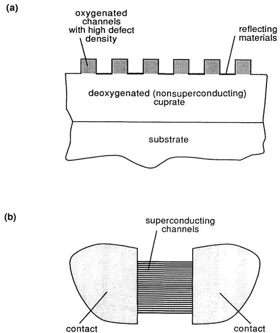
FIG. 5. Proposed superconductor detector configuration: (a) cross section, (b) general view.
