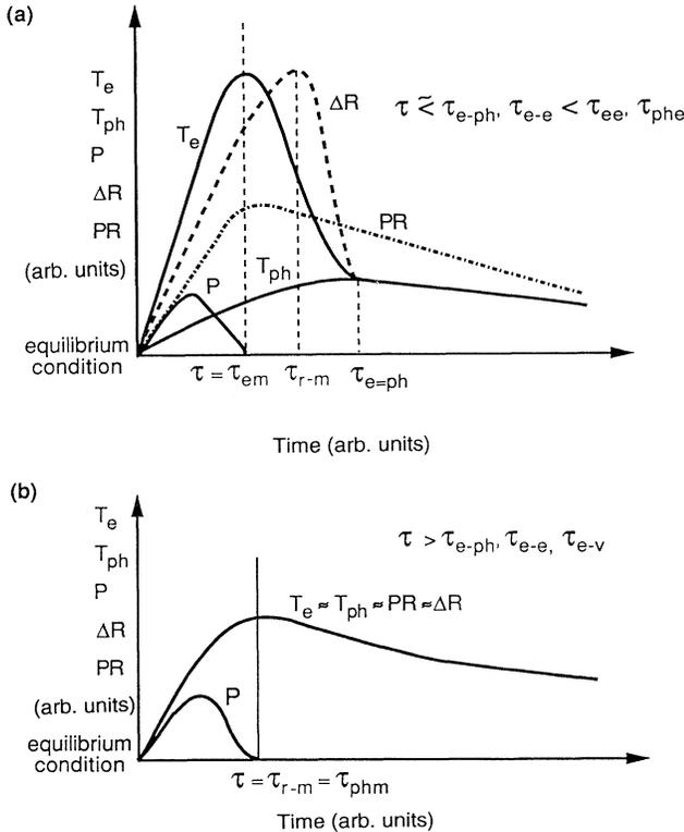
FIG. 3. Nonequilibrium dynamic behavior in a superconductor for two extreme cases: (a)  $\tau < \tau_{e-ph}$ ,  $\tau_{e-e} < \tau_{ee}$ ,  $\tau_{ph}$ ; (b)  $\tau > \tau_{e-ph}$ ,  $\tau_{e-e}$ ,  $\tau_{e-v}$ ;  $T_e$  is the electron temperature,  $T_{ph}$  is the phonon temperature,  $P$  is the optical pulse, PR is the photoresponse,  $\Delta R$  is the reflectivity response.
