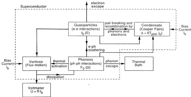
FIG. 1. Block diagram of a superconductor for an equilibrium condition before the optical pulse.
