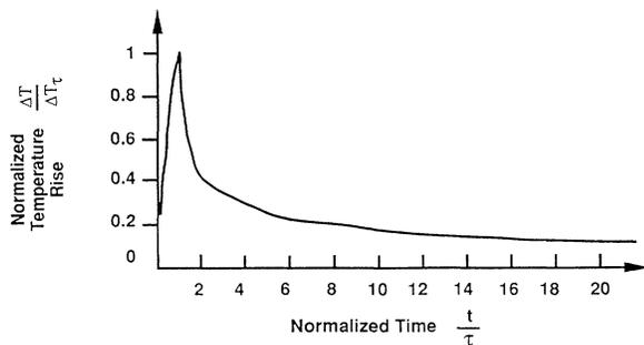
FIG. 4. The dependence of the normalized temperature rise  $\Delta T/\Delta T_\tau$  as a function of the normalized time normalized to the laser pulse duration  $\tau$  [from Frenkel *et al.* (Ref. 7)].
