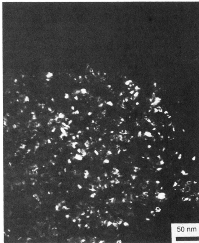
FIG. 6. (a) Bright-field and (b) dark-field TEM micrographs from sample N2 indicating the presence of a bimodal grain-size distribution. Grains with an average size of approximately 8 nm are seen in the lower portion of the figures, while micrometer-sized grains are seen in the upper portion of the figures.
