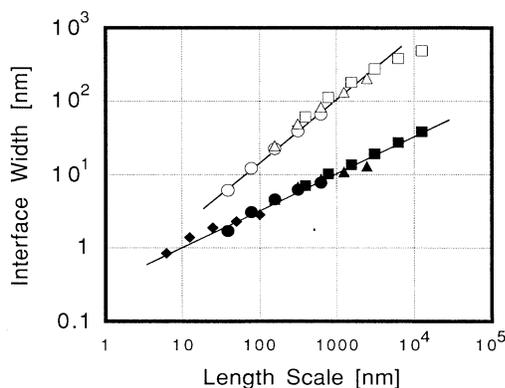
FIG. 2. Interface width  $w$  vs surface-size  $r$  plot for the surface *A* (solid marks) and *B* (open marks). The plots are for  $50 \times 50$  (squares),  $20 \times 20$  (triangles), and  $5 \times 5$  (circles)  $\mu\text{m}^2$  measured areas for the same central point by AFM and for  $0.8 \times 0.8$  (diamonds)  $\mu\text{m}^2$  by STM for the same sample. Solid lines of slopes  $\frac{1}{2}$  and 0.87 are drawn as guides to the eye.
