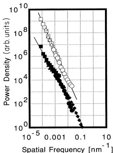
FIG. 3. Surface power spectral density vs spatial frequency for the same surface topographs used in Fig. 2. Solid lines of slopes 2 and 2.5 are drawn as guides to the eye.
