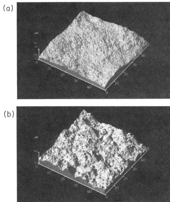
FIG. 1. AFM topographs of the copper electrodeposits of  $50\text{-}\mu\text{m}$  thickness: (a) for sample *A* and (b) for sample *B*. The vertical scale is greatly expanded in (a). All lengths are in  $\mu\text{m}$ .
