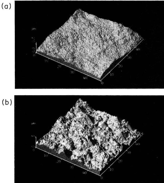
FIG. 1. AFM topographs of the copper electrodeposits of 50- $\mu\text{m}$  thickness: (a) for sample *A* and (b) for sample *B*. The vertical scale is greatly expanded in (a). All lengths are in  $\mu\text{m}$ .
