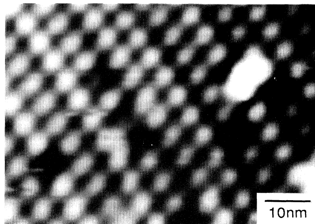
FIG. 2. A well-ordered p(2 \times 2) sulfur overlayer ( 3 \text{ V}/1 \text{ nA} ).
