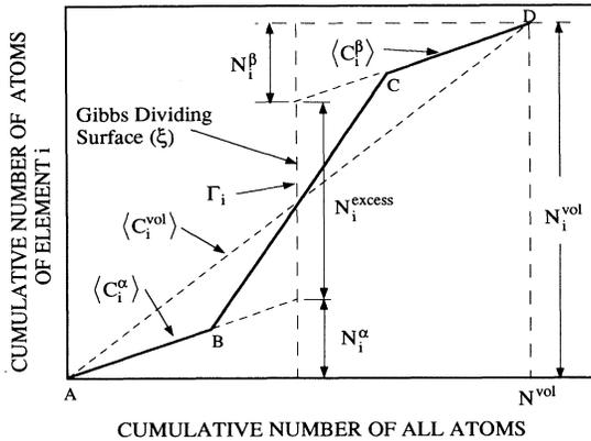
FIG. 2. Hypothetical integral profile (line ABCD) showing how the excess number of solute atoms is determined from an APFIM analysis of a volume of material as in Fig. 1.
