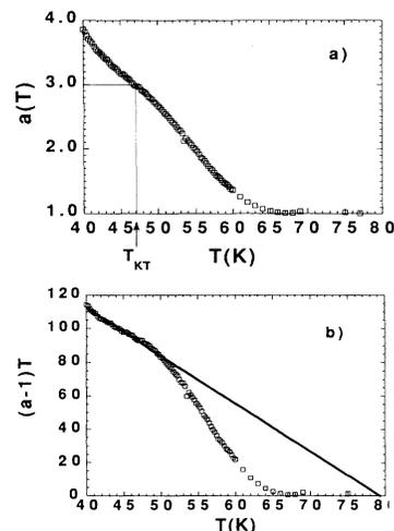
FIG. 4. From the  $I$ - $V$  data in Fig. 3, (a) the power-law coefficient  $a(T)$  and (b) the expression  $[a(T)-1]T$  are plotted vs  $T$ , showing how  $T_{KT}$  and  $T_{c0}$  are determined.
