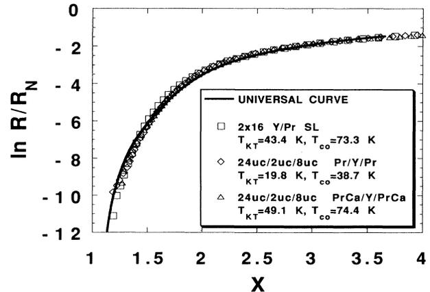
FIG. 2. Normalized resistance vs the scaling variable  $X$  for the three structures considered in Fig. 1.
