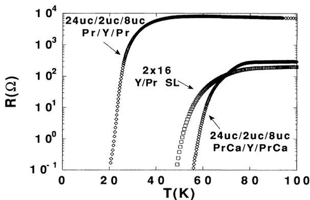
FIG. 1. Resistance plotted against temperature for three structures containing two unit-cell-thick YBCO layers.
