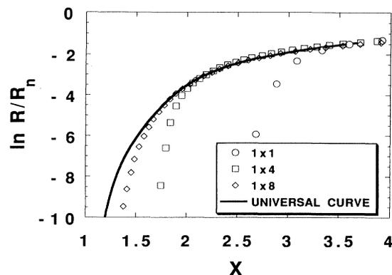
FIG. 5. Normalized resistance vs the scaling variable ( $X$ ) for a series of  $1 \times N$   $\text{YBa}_2\text{Cu}_3\text{O}_{7-\delta}/\text{Pr}_{0.5}\text{Ca}_{0.5}\text{Ba}_2\text{Cu}_3\text{O}_{7-\delta}$  superlattice structures. The anisotropic, 3D layered superconductor shows progressively larger departures from the universal resistance curve for a quasi-2D superconductor, as interlayer coupling is increased.
