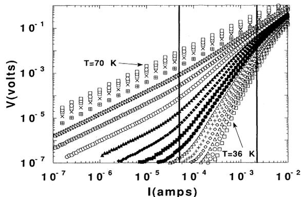
FIG. 3.  $I$ - $V$  characteristics measured at temperatures ranging from 36 to 70 K for the 24uc/2uc/8uc  $\text{Pr}_{0.5}\text{Ca}_{0.5}\text{Ba}_2\text{Cu}_3\text{O}_{7-\delta}/\text{YBa}_2\text{Cu}_3\text{O}_{7-\delta}/\text{Pr}_{0.5}\text{Ba}_2\text{Cu}_3\text{O}_{7-\delta}$  structure. The vertical lines show the approximate boundaries of the low- and high-current behavior discussed in the text.
