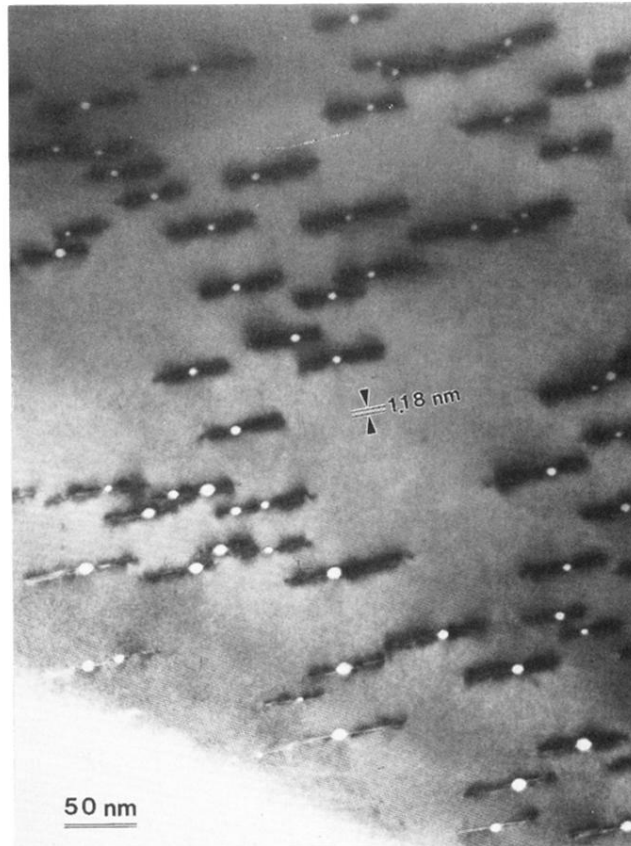
FIG. 13. (100) lattice image of \text{YBa}_2\text{Cu}_3\text{O}_{7-\delta} ( \delta < 0.1 ) irradiated with Ag ions showing stacking faults, viewed edge on, created by the radiation damage. The stacking faults are seen as dark wide lines in thick region and white narrow lines in thin region.
