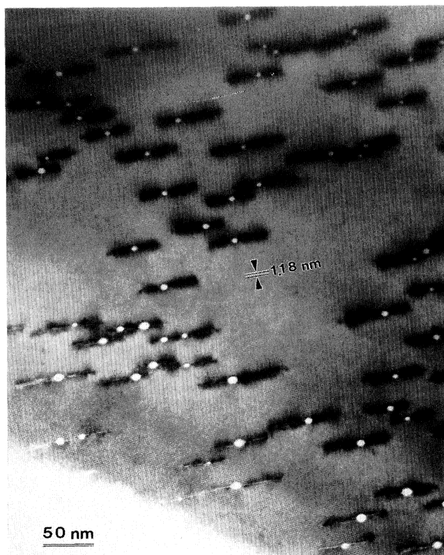
FIG. 13. (100) lattice image of \text{YBa}_2\text{Cu}_3\text{O}_{7-\delta} ( \delta < 0.1 ) irradiated with Ag ions showing stacking faults, viewed edge on, created by the radiation damage. The stacking faults are seen as dark wide lines in thick region and white narrow lines in thin region.
