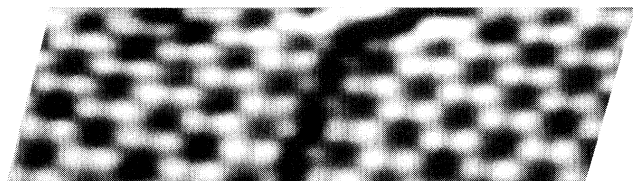
FIG. 4. STM image of an antiphase boundary in the trimer \sqrt{3} \times \sqrt{3} phase. This image is about 20 \text{ \AA} \times 50 \text{ \AA} and has been corrected for thermal drift. V_t = -0.82 V, I_t = 0.11 nA.
