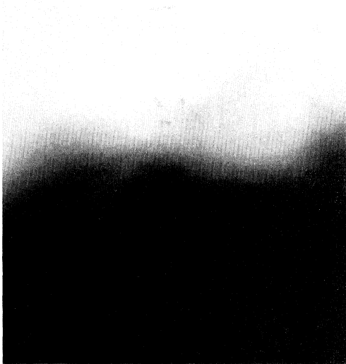
FIG. 3. Image of the phonon-induced voltages across the contacts 2/3 in a magnetic field of about 4.5 T. The Fermi energy is in the lower half of a Landau level. The large diffuse areas (bright at top, dark at bottom) are due to the Nernst-Ettingshausen effect. A ballistic phonon-drag image is superimposed on this image but is hardly visible in the reproduction.
