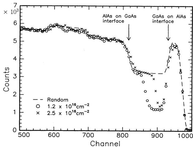
FIG. 1. Backscattering spectra of a 1.0-MeV Kr irradiated GaAs/AlAs/GaAs trilayer sample in the  $\langle 100 \rangle$  channeling direction after fluences of  $1.2 \times 10^{16} \text{ cm}^{-2}$  ( $\circ$ ), and  $2.5 \times 10^{16} \text{ cm}^{-2}$  ( $\times$ ). A random spectrum (---) is included for comparison.
