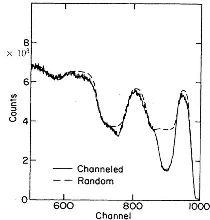
FIG. 2. Backscattering spectrum of a 1.0-MeV Kr irradiated GaAs/AlAs/GaAs/AlAs/GaAs pentalayer sample in the  $\langle 100 \rangle$  channeling direction after a fluence of  $1 \times 10^{16} \text{ cm}^{-2}$ . A random spectrum (---) is included for comparison.
