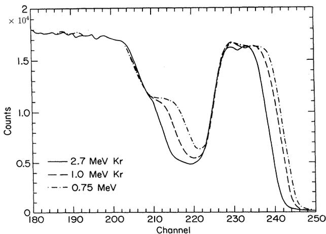
FIG. 3. Backscattering spectra of a GaAs/AlAs/GaAs tri-layer sample in the  $\langle 100 \rangle$  channeling direction after irradiation with 0.75-, 1.0-, or 2.7-MeV Kr ions. The doses are normalized to produce the same damage energy at the back interface.
