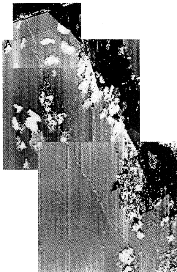
FIG. 1. Large-scale images of the superlattice (lower right) and its boundary with normal graphite region (upper left). These images are taken with set current 2.3 nA and tip bias 490 mV. The size of the left bottom square is a 4000 \times 4000 \text{ \AA}^2 . The gray-scale range is 3 \text{ \AA} . The hexagonal superstructure has a periodicity of 65.8 \text{ \AA} .
