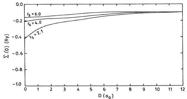
FIG. 5. Self-energy of an electron at zero speed placed at the center between two metal surfaces as a function of gap width with dispersion effects included.
