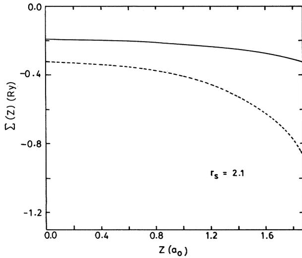
FIG. 1. Self-energy of an electron with zero speed as a function of distance between the gap of two metal surfaces for  $r_s = 2.1$ . The solid and the dashed curves are with dispersion included and excluded, respectively.
