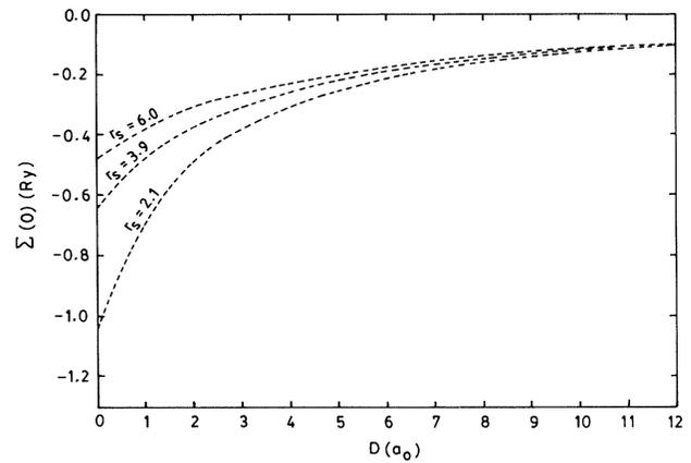
FIG. 4. Self-energy of an electron at zero speed placed at the center between two metal surfaces as a function of gap width with dispersion effects excluded.
