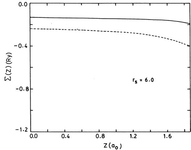
FIG. 3. Self-energy of an electron with zero speed as a function of distance between the gap of two metal surfaces for  $r_s = 6.0$ . The solid and the dashed curves are with dispersion included and excluded, respectively.
