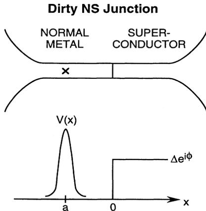
FIG. 1. Impurity potential  $V(x)$  and pair potential  $\Delta(x)$  used in this calculation. The point defect  $V(x)$  can be located either in the superconductor or normal conductor.
