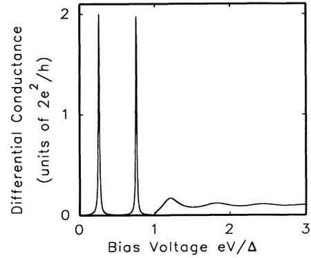
FIG. 2. Differential conductance for a NINS geometry, formed when the impurity resides in the normal metal ( $L = 100$  nm). Each subgap ( $eV < \Delta$ ) transmission resonance corresponds to an additional quasiparticle trapped between the impurity and superconductor.
