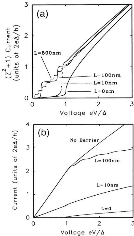
FIG. 3. Current-voltage characteristics of the SN junction when the impurity is (a) in the normal metal and (b) inside the superconductor. A large subgap current, due to conduction through resonant quasiparticle states, flows when the impurity is located in the normal metal. When the impurity is several coherence lengths inside the superconductor, the current reaches its ballistic value for  $eV < \Delta$ , but is limited by reflections from the impurity when  $eV > \Delta$ .
