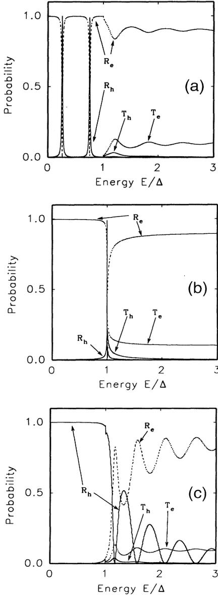
FIG. 5. Transmission coefficients versus energy, when the impurity is (a) in the normal metal ( $L = 100$  nm), (b) at the SN interface ( $L = 0$  nm), and (c) inside the superconductor ( $L = 100$  nm). The oscillating transmission arises from quasi-bound states forming between the impurity and SN interface.
