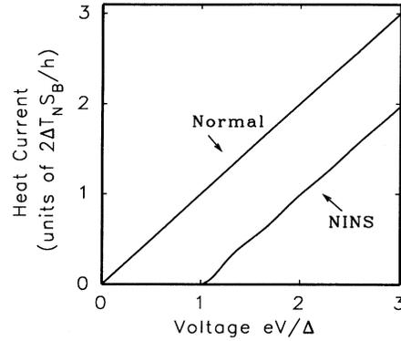
FIG. 4. Heat current flow in an NINS junction (having  $L = 100$  nm) compared to the heat current flow in the normal state (NIN). Heat currents are completely suppressed by Andreev reflections inside the superconducting gap, producing a heat current deficit for  $eV \gg \Delta$ .
