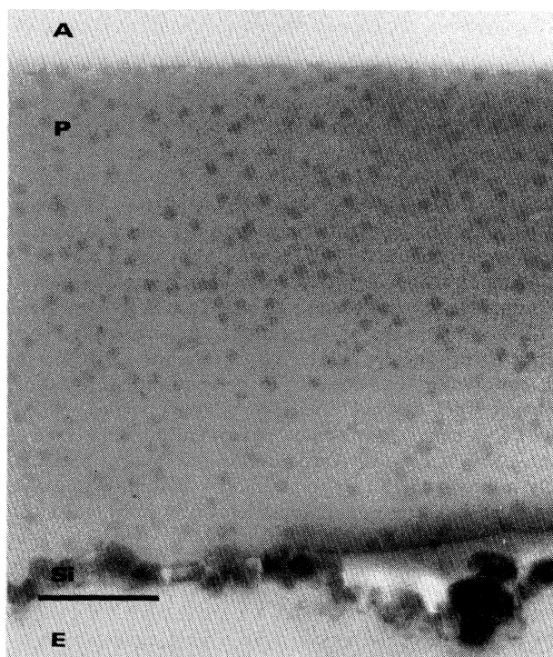
FIG. 1. Cross-sectional view of a 15 wt % 75–102 k dPS-P2VP in 190 k hPS. Annealing time is 52 h at 180 °C. Layer thickness is 2000 nm. The micellar surface layer is clearly visible. (Bar indicates 400 nm, A=air, P=polymer layer, Si=silicon layer, E=epon substrate.)
