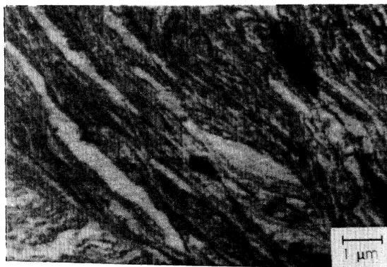
FIG. 3. Cross section of an etched  $\text{Cu}_{50}\text{Co}_{50}$  powder blend mechanically alloyed for 20 h.
