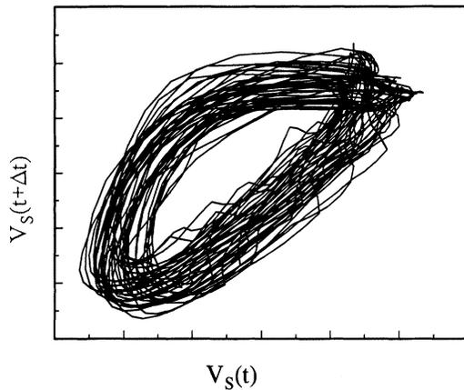
FIG. 3. Phase portrait of the quasiperiodic voltage signal of Fig. 2 constructed via the time-delay method ( $\Delta t = 0.48$  ms).
