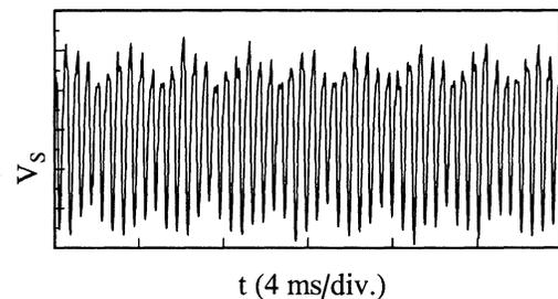
FIG. 2. Temporal structure of the self-generated quasiperiodic voltage signal obtained at the constant parameters time-averaged voltage  $\bar{V}_S = 2.178$  V, current  $I_S = 2.527$  mA, transverse magnetic field  $B = 11.5$  G, and temperature  $T = 2.1$  K.
