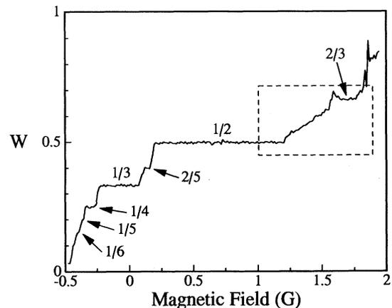
FIG. 11. Winding number as a function of the transverse magnetic field obtained from the data of Fig. 10. The dashed rectangular area is magnified in Fig. 12.
