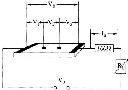
FIG. 1. Schematic illustration of the experimental setup. The dark areas on the surface of the semiconductor sample indicate the ohmic contacts.
