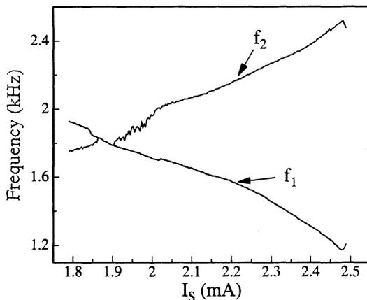
FIG. 4. Development of the two fundamental intrinsic frequencies under variation of the sample current obtained at the constant parameters  $\bar{V}_S = 2.15$  V,  $B = 10.0$  G, and  $T = 1.8$  K.
