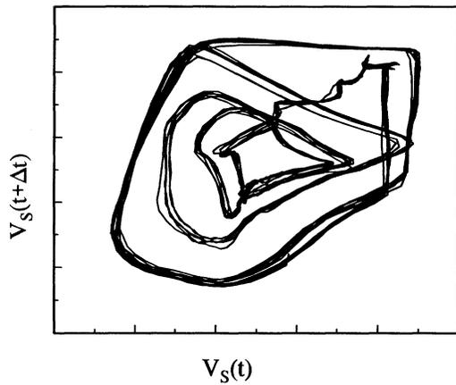
FIG. 8. Phase portrait of the mode-locked voltage signal of Fig. 6 constructed via the time-delay method ( $\Delta t = 0.24$  ms).
