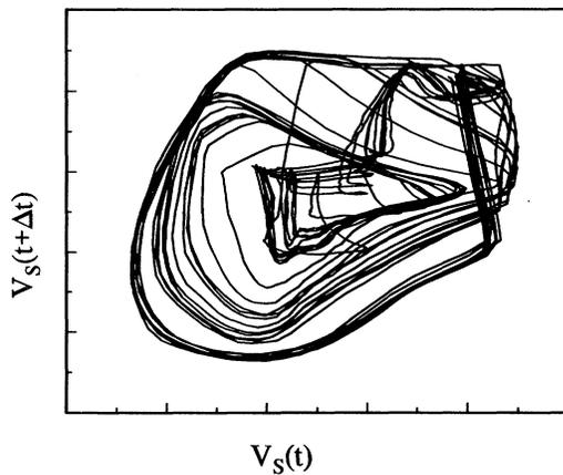
FIG. 9. Phase portrait of the quasiperiodic voltage signal obtained at the constant parameters  $\bar{V}_S = 2.21$  V,  $I_S = 2.53$  mA,  $B = -0.38$  G, and  $T = 2.01$  K ( $\Delta t = 0.24$  ms).
