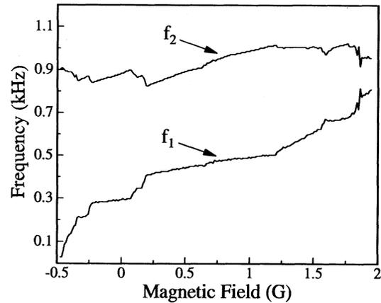
FIG. 10. Development of the two fundamental intrinsic frequencies under variation of the transverse magnetic field obtained at the constant parameters  $\bar{V}_S = 2.21$  V,  $I_S = 2.53$  mA, and  $T = 2.01$  K.
