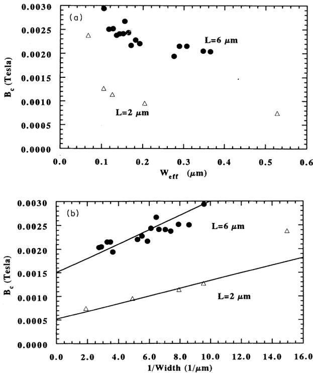
FIG. 3. (a) The experimentally observed variation of  $B_c$  with channel width in both the 2- and 6- $\mu\text{m}$  channels. (b) The data of (a) replotted to show the approximately inverse relationship between  $B_c$  and  $W_{\text{eff}}$ .
