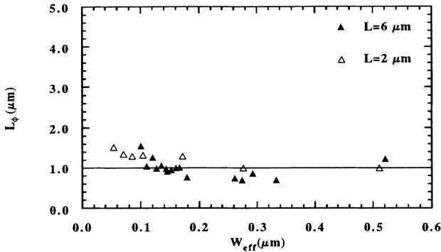
FIG. 2. The width dependence of the phase coherence length in the 6- and 2- $\mu\text{m}$  length channels. The value of  $l_\phi$  was derived by fitting Eq. (3) to the experimentally observed NMR, and is seen to be essentially independent of channel width and length.
