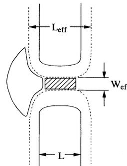
FIG. 4. Presumed form of the actual sample geometry, consisting of a confined region  $A$ , associated with the split metal gates, and an unconfined region  $B$ , which extends into the 2DEG. Since  $l_\phi$  is comparable to  $L$ , electrons in region  $A$  will in some sense be nonlocally influenced by electrons in region  $B$ .
