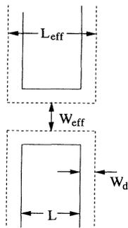
FIG. 1. Schematic diagram of the depletion layer induced around the gate edges by the negative bias. The solid line represents the actual gate geometry, while the dashed line represents the extent of the depletion layer. In reality, electron screening will round the corners and our assumption of a “hard-wall potential” will be only approximate.
