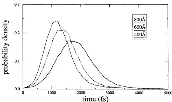
FIG. 3. The electron density  $\rho$  inside the junction region  $\Omega=VI+VII+V$  vs time  $t$  (fs). Parameters:  $a = L = 100 \text{ \AA}$ ,  $b = 440 \text{ \AA}$ ,  $k_0a = 0.6$ , and  $V_0 = 4.54 \text{ meV}$ . Here the solid line, dotted line, and dashed line correspond to the spatial spread of incoming electron wave packet  $\sigma = 800 \text{ \AA}$ ,  $600 \text{ \AA}$ , and  $500 \text{ \AA}$ , respectively.
