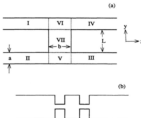
FIG. 1. (a) Schematic view of the four-terminal electron waveguide coupler where regions VI, VII, and V form the interaction region. (b) Schematic view of a quantum wire with a narrow double constriction.
