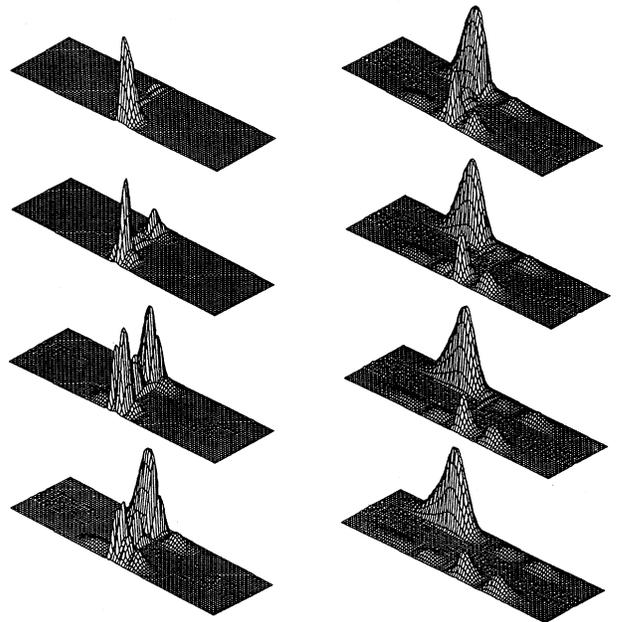
FIG. 2. Time evolution of the electron wave packet for every 1000 time steps on the electron waveguide coupler. The figures are ordered according to time from up to down and left to right. Over 60% of the electron wave has been transferred. Parameters:  $a = L = 100$  Å,  $b = 440$  Å,  $\sigma = 300$  Å,  $k_0 a = 0.8$ ,  $V_0 = 4.54$  meV, and the time step is 0.23 fs.
