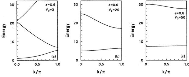
FIG. 2. The first two minibands of the energy spectrum (in units of  $\hbar^2/ma_0^2$ ) of a superlattice with well width of  $a = 0.6$  and potential strength: (a)  $V_0 = 3$ , (b)  $V_0 = 20$ , and (c)  $V_0 = 50$ .
