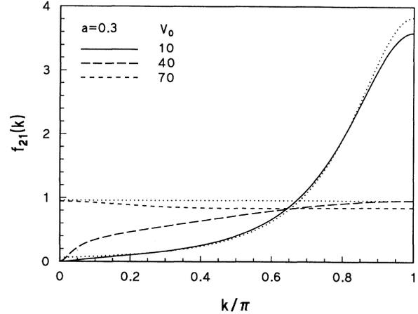
FIG. 6. The oscillator strength  $f_{21}(k)$  as function of the electron wave vector for a well width of  $a = 0.3$  and three different values of the height of the potential barrier. The results for  $V_0 \rightarrow 0$  and for a single quantum well are given by the dotted curves.
