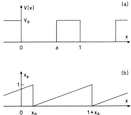
FIG. 1. (a) Superlattice potential and (b) periodic coordinate operator in dimensionless units.
