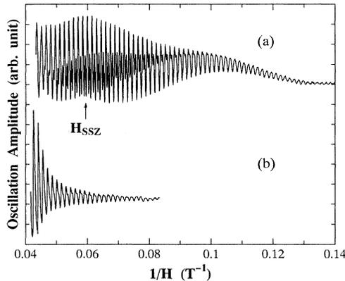
FIG. 1. Splitting wave form of SdH (a) and dHvA (b) oscillations at 0.5 K in the field perpendicular to the plane.
