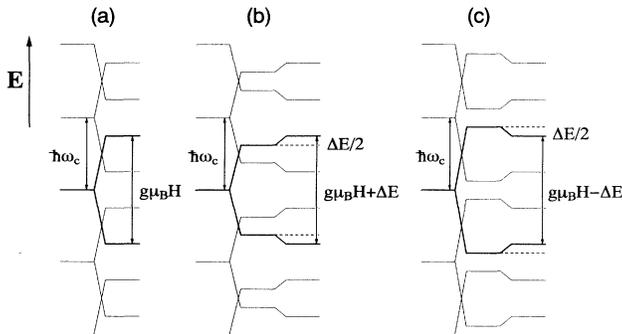
FIG. 5. Electron energy levels in a magnetic field; (a)  $J = 0$ , (b)  $J > 0$ , and (c)  $J < 0$ .
