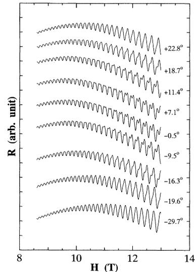
FIG. 3. Field orientation dependence of SdH oscillations at 0.5 K. The angle shown in the figure is measured from the perpendicular direction to the conducting plane.
