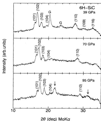
FIG. 2. X-ray-diffraction patterns recorded for 6H-SiC. Only Mo  $K\alpha$  radiation was employed. G denotes reflection from the gasket. The peaks labeled by arrows are reflections other than from 6H phase.
