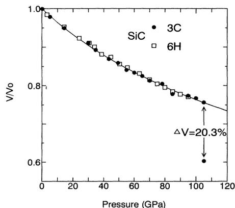
FIG. 3. Change of the relative volume of 3C and 6H polytypes of SiC as a function of pressure.
