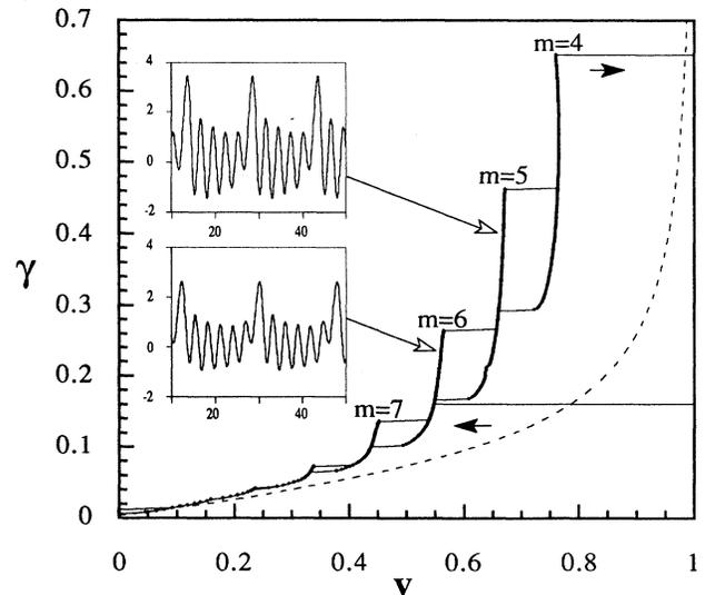
FIG. 1.  $IV$  characteristics of the 1D annular Josephson-junction array with the parameters  $N = 10$ ,  $a = 1.0$ , and  $\alpha = 0.1$ . Solid arrows indicate the direction of switching in the hysteresis loop. The dashed line shows the  $IV$  curve for the continuum case calculated for the system with the same normalized length. The insets show the voltage evolution for two different points of the  $IV$  curve measured in the middle point of the array.
