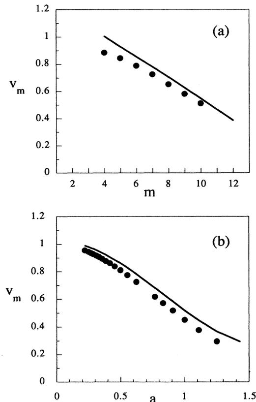
FIG. 2. The voltage position of the discreteness-induced resonances  $v_m$  as a function of the resonance number  $m$  for  $a = 0.625$  (a) and of the array spacing  $a$  for  $m = 7$  (b). Squares correspond to the numerical results; the solid line is given by Eq. (7).
