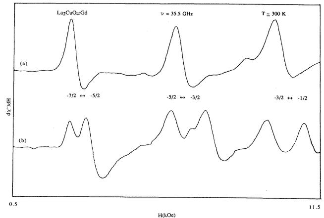
FIG. 3. Low-field  $\text{La}_2\text{CuO}_4\text{:Gd}$  EPR spectra at  $T = 300$  K ( $> T_0$ ) for (a)  $\mathbf{H}_0 \parallel b$  axis, (b)  $\mathbf{H}_0$  at  $25^\circ$  from the  $b$  axis in a plane containing the  $[101]$  axis.
