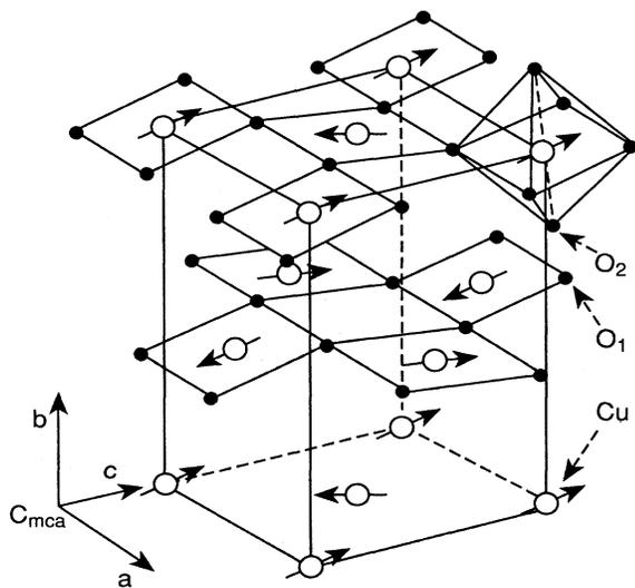
FIG. 2. Orthorhombic structure (space group  $Cmca$ ) of  $\text{La}_2\text{CuO}_4$ . The  $\text{CuO}_6$  octahedra are staggered tilt by  $\sim 4^\circ$  and the Cu spins canted from the  $\text{CuO}$  planes by  $\sim 0.2^\circ$  according to the neutron data (from Ref. 4).
