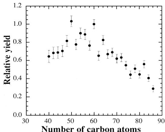
FIG. 4. Yield of carbon-cluster ions desorbed from a PVDF target as a function of number of atoms in the cluster.
