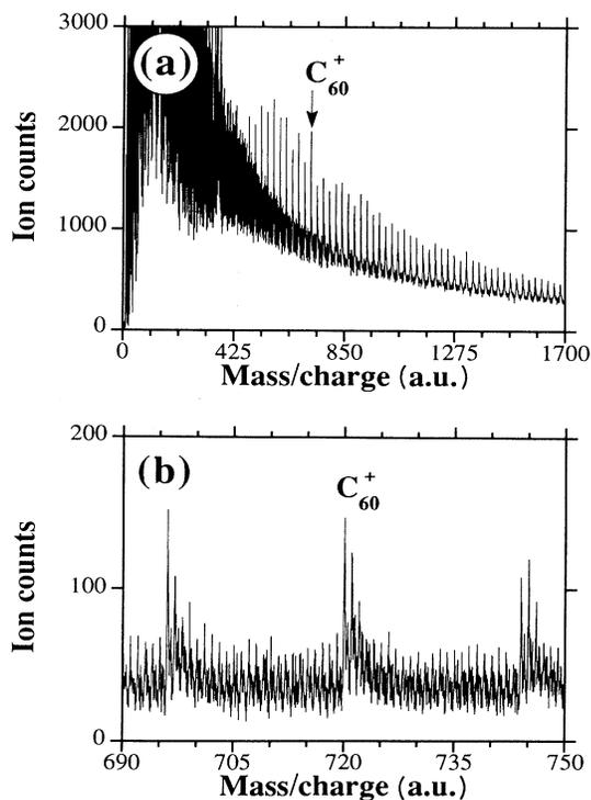
FIG. 3. (a) A time-of-flight (reflected mode) spectrum of positive cluster ions from a PVDF target in the  $m/q$  range from 0 to 1700 a.u. (b) Expanded region from the same spectrum in the  $m/q$  range from 690 to 750 a.u.
