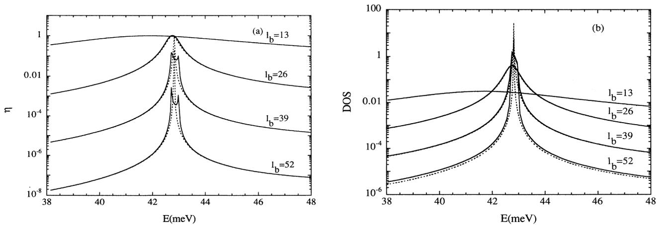
FIG. 3. Effect of alloy disorder on (a) the barriers on the transmission coefficients and (b) the DOS in the well region for structures with the same disorder strength ( $P_A=0.15$ ,  $\nu_A=8.5$  meV,  $V_{\text{off}}=120$  meV) and the same well width ( $l_w=24$  monolayers) but different barrier widths,  $l_b=13, 26, 39, 52$  monolayers from top to bottom. The results for disorder-free structures are also plotted with the dotted line for comparison.
