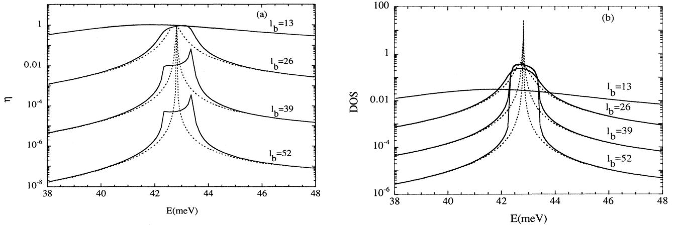
FIG. 4. Effect of alloy disorder inside the well on (a) the transmission coefficients and (b) the DOS in the well region for structures with the same disorder strength ( $P_A = 0.15$ ,  $v_A = 8.5$  meV,  $V_{\text{off}} = 120$  meV) and the same well width ( $l_w = 24$  monolayers) but different barrier widths,  $l_b = 13, 26, 39, 52$  monolayers from top to bottom. The results for disorder-free structures are also plotted with the dotted line for comparison.
