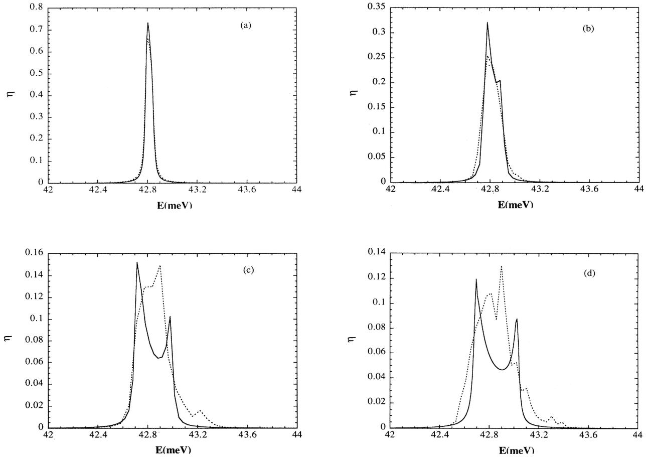
FIG. 2. Transmission coefficients calculated from the CPA method (solid line) compared with numerical simulation (dotted line) for DBQW structures with different disorder strength in the barriers:  $P_A=0.15$ ,  $\nu_A=(a)$  1.7 meV, (b) 4.25 meV, (c) 8.5 meV, and (d) 10.2 meV. Structural parameters:  $V_{\text{off}}=120$  meV, the width of the barriers and the well are 39 and 24 (in units of monolayer width), respectively.
