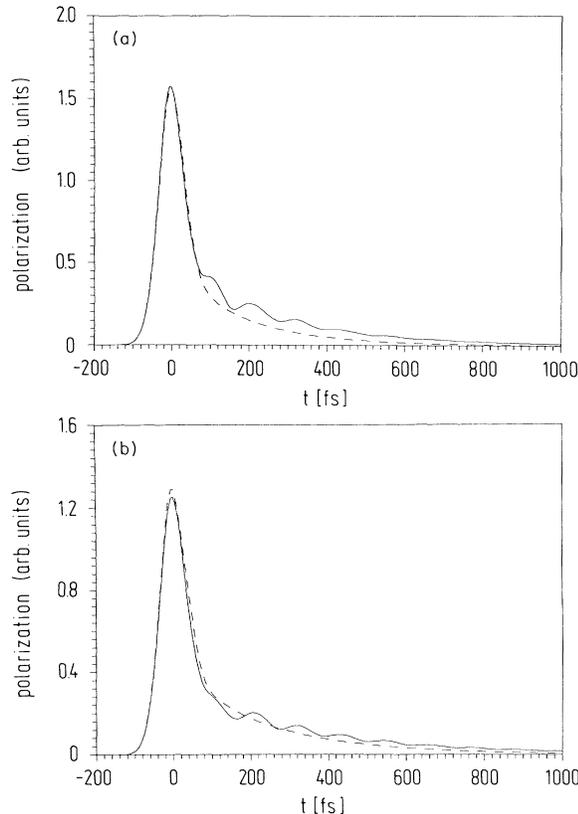
FIG. 7. Incoherently summed polarization  $P(t) = \sum |P_k(t)|$  vs time for InP excited with a 50-fs pulse peaking at  $t=0$  with an excess energy of (a) 60 meV and (b) 20 meV, and a Rabi frequency of  $dE_0 = 26.4$  meV. Full line: with memory; long-dashed line: without memory.
