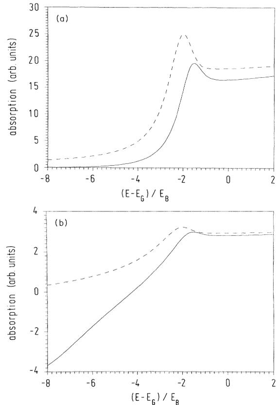
FIG. 8. Linear band-tail absorption spectrum of GaAs at room temperature. Full line: with memory; long-dashed line: without memory. (a) On a linear scale, (b) on a logarithmic scale.
