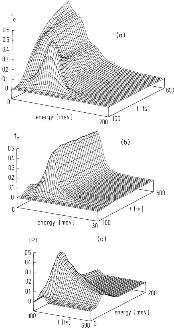
FIG. 1. Distributions (a)  $f_{ke}(t)$  and (b)  $f_{kh}(t)$  and absolute amount of the interband polarization (c)  $|P_k(t)|$  vs energies  $e_{ke}$ ,  $e_{kh}$ , and  $e_{ke}$ , respectively, and time for GaAs excited with a 50-fs pulse peaking at  $t=0$  with 60-meV excess energy and a Rabi frequency of  $dE_0 = 13.2$  meV.
