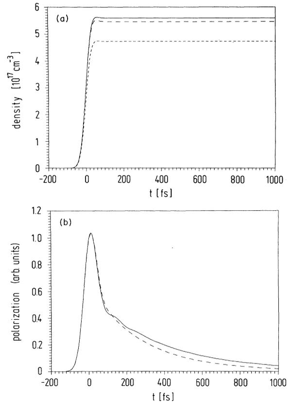
FIG. 2. (a) Total  $e$ - $h$  density and incoherently summed polarization (b)  $P(t) = \sum |P_k(t)|$  vs time for GaAs excited with a 50-fs pulse peaking at  $t=0$  with 60-meV excess energy and a Rabi frequency of  $dE_0 = 13.2$  meV. Full line: with memory; long-dashed line: without memory; short-dashed line: with memory but without excitonic effects.
