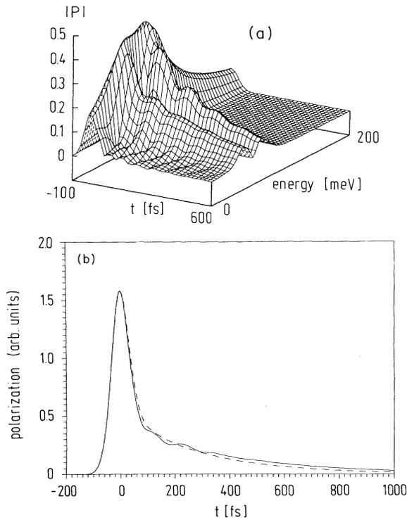
FIG. 3. Absolute amount of (a) the interband polarization  $|P_k(t)|$  versus energy  $e_{ke}$  and time and (b) the incoherently summed polarization  $P(t) = \sum |P_k(t)|$  vs time for GaAs excited with a 50-fs pulse peaking at  $t=0$  with 60-meV excess energy and a Rabi frequency of  $dE_0 = 26.4$  meV. Full line: with memory; long-dashed line: without memory.
