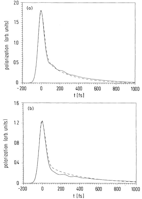
FIG. 4. Incoherently summed polarization  $P(t) = \sum |P_k(t)|$  vs time for GaAs excited with a 50-fs pulse peaking at  $t=0$  with an excess energy of (a) 100 and (b) 20 meV, and a Rabi frequency of  $dE_0 = 26.4$  meV. Full line: with memory; long-dashed line: without memory.
