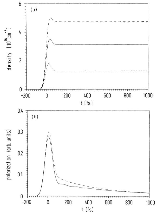
FIG. 6. (a) Total  $e$ - $h$  density and (b) incoherently summed polarization  $P(t) = \sum |\mathbf{P}_k(t)|$  vs time for GaAs excited with a 50-fs pulse peaking at  $t=0$  for nonresonant excitation 10 meV below the gap and a Rabi frequency of  $dE_0 = 6.6$  meV. Full line: with memory; long-dashed line: without memory; short-dashed line: with memory but without excitonic effects.
