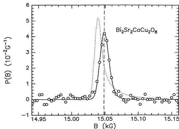
FIG. 3. Spectrum for  $\text{Bi}_2\text{Sr}_2\text{CaCu}_2\text{O}_{8+\delta}$  crystals with  $H$  (dashed line) along  $c$ . Solid curve is a fit using a disordered 2D fluxon model. The dotted curve is for a perfect triangular lattice.  $\lambda_{ab} = 2500$  Å for both curves.
