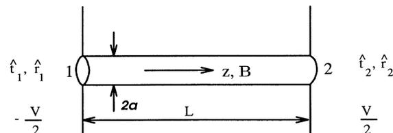
FIG. 1. A ballistic microwire modeled as cylindrical channel between two large electron reservoirs. The *probabilities* for scattering at contact 1 (2) between modes in the reservoir and the channel (transmission) or between modes in the reservoir (reflection) are given by the elements of the matrices  $\hat{t}_{1(2)}$  and  $\hat{r}_{1(2)}$ .
