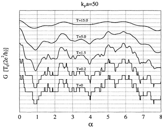
FIG. 3. Conductance as a function of normalized magnetic flux through the microwire. Results are shown for  $T=0, 0.2, 1.5, 5.0,$  and  $15.0$  (in units of  $\hbar^2/m^*a^2k_B$ ). At temperatures below unity in these units, sharp fluctuations appear on the scale of only a fraction of a flux quantum  $\phi_0$ ; a new scale for mesoscopic phenomena. At higher temperatures only smooth conductance oscillations on the scale of  $\phi_0$  remain. All curves were calculated for  $k_F a = 50$ .
