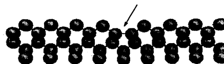
FIG. 2. The structure of the \text{Ge}_n\text{Si}(001) (2 \times N) surface projected onto the [011] plane. The arrow marks the position of the missing dimer. Note that the second-layer atoms have shifted to form a bond.
