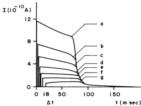
FIG. 1. Current traces obtained with the SRT, for varying pausing times  $\Delta t$ , which is the time elapsed between the flash and the application of the electric field. The values of  $\Delta t$  are 0.41 ms (curve *a*), 1.45 ms (*b*), 3.9 ms (*c*), 5.5 ms (*d*), 7.8 ms (*e*), 11.5 (*f*), and 18 ms (*g*). The origin of the time scale corresponds to the instant the light was flashed. Note the monotonic decrease of the current and the common long-lived tail in the traces.
