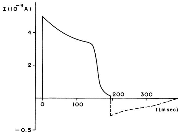
FIG. 2. Current traces with the IFT, where the inversion of the field was performed after the main transit of the normal carriers. Note that the scale of the dashed return (negative) current is four times enlarged, and the dispersive trend of the reversed signal.
