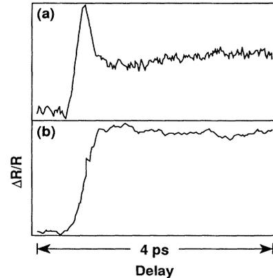
FIG. 5. Normalized  $\Delta R/R$  ( $\sim 10^{-3}$ ) measured on the YBCO-I sample at  $T=12$  K using a 2-eV probe photon energy. The pump intensity was (a)  $\sim 20 \mu\text{J}/\text{cm}^2$  and (b)  $\sim 100 \mu\text{J}/\text{cm}^2$ .
