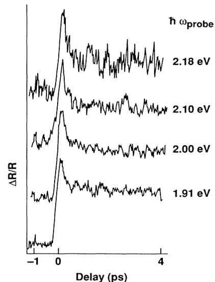
FIG. 1. Normalized changes in reflectivity  $\Delta R/R$  ( $\sim 10^{-4}$ ) measured on the YBCO-III (oxygen-rich) sample at room temperature using the probe photon energies indicated in the figure.
