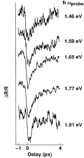
FIG. 2. Normalized changes in reflectivity  $\Delta R/R$  ( $\sim 10^{-3}$ ) measured on the YBCO-VI (oxygen-poor) sample at room temperature using the probe photon energies indicated in the figure.
