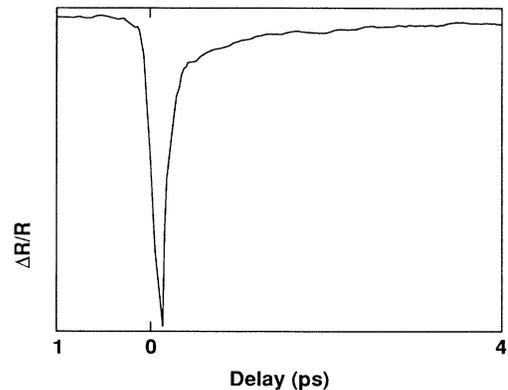
FIG. 3. Normalized  $\Delta R/R$  measured on the YBCO-V (partially oxygen depleted) sample at room temperature using a 2-eV probe photon energy.
