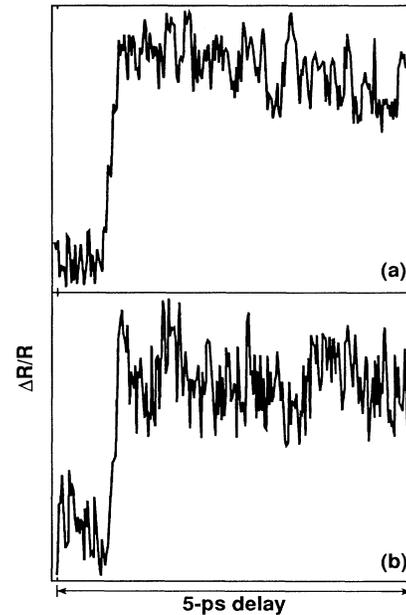
FIG. 7. Normalized  $\Delta R/R$  measured with a 2-eV probe on the YBCO-II microbridge biased by the following levels of electric current: (a) 0 and (b) 15 mA. The critical current of the microbridge was 12 mA. The temperature was about 79 K and the pump intensity was  $\sim 100 \mu\text{J}/\text{cm}^2$ .
