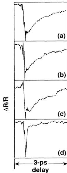
FIG. 6. Normalized  $\Delta R/R$  measured with a 2-eV probe on the YBCO-IV microbridge biased by the following levels of electric current: (a) 0, (b) 1.5 mA, (c) 6 mA, and (d) 10 mA. The critical current of the microbridge was 8 mA. The temperature was about 72 K and the pump intensity was  $\sim 1 \mu\text{J}/\text{cm}^2$ .
