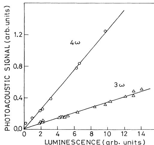
FIG. 6. Direct comparison of the photoacoustic and luminescent signals simultaneously generated after  $3\omega$  and  $4\omega$  excitation.
