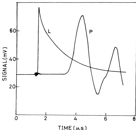
FIG. 3. Temporal response of the luminescent ( $L$ ) and photoacoustic ( $P$ ) signals.
