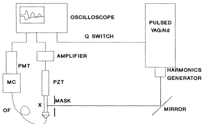
FIG. 1. Experimental setup used for the simultaneous measurement of photoacoustic and luminescent signals. PMT, photomultiplier tube; MC, monochromator; OF, optical fiber; PZT, piezoelectric transducer; and X, crystal.
