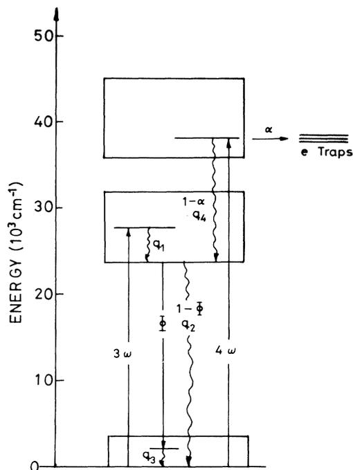
FIG. 5. Schematic energy diagram indicating the different contributions to the photoacoustic and luminescent signals.
