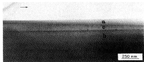
FIG. 2. TEM bright-field image of a cross section of self-implanted Si during heating in situ at 540^\circ\text{C} . The arrow indicates the direction along which the thickness of the specimen decreases. (a) amorphous layer, (c) epitaxially grown crystalline layer, (b) bulk crystal. The effect of the reduced SPE rate in the thinner region is evident.
