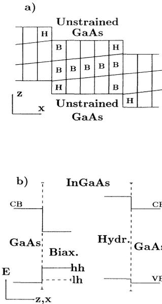
FIG. 3. (a) Schematic representation of the lattice deformation of an  $\text{In}_x\text{Ga}_{1-x}\text{As}/\text{GaAs}$  QW. The  $H$  and  $B$  mean zones under hydrostatic and biaxial strain, respectively. (b) Band lineup in the  $H$  and  $B$  zones.
