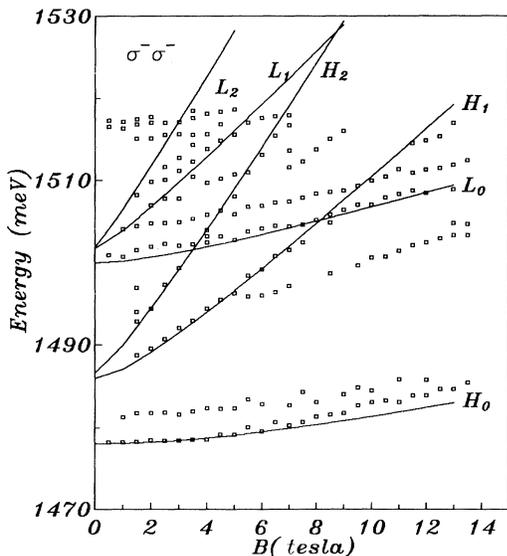
FIG. 2. PLE transition energies at 2 K as a function of magnetic field. Continuous lines fit the data to a two-dimensional hydrogenic magnetoexciton (see text).
