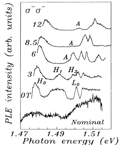
FIG. 1. Photoluminescence excitation (PLE) spectra at 2 K of a 15-Å-thick quantum well (QW) grown on a vicinal substrate for selected values of the applied magnetic field,  $B$ . Spectra have been offset vertically for clarity. A spectrum from the nominal sample at 0 T is also shown for comparison.
