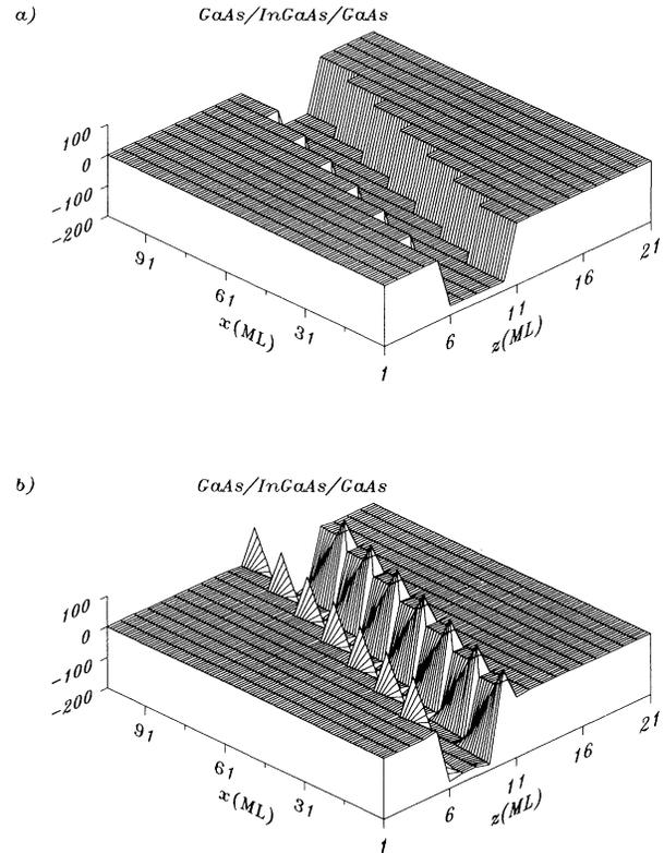
FIG. 4. 3D plot of the conduction-band profile, in the  $x, z$  plane, of a 15-Å thick  $\text{InGaAs}/\text{GaAs}$  vicinal QW with 40-Å long terraces taking into account (a) stepped interfaces and homogeneous biaxial stress within the well, and (b) including inhomogeneous strain. Each node in the plot represents a cell. The origin of energies has been taken at the GaAs barrier conduction band.
