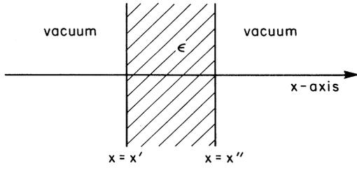
FIG. 1. The geometry of a single dielectric slab of dielectric constant  $\epsilon$  surrounded by a vacuum. Left face at  $x = x'$  and right face at  $x = x''$ .
