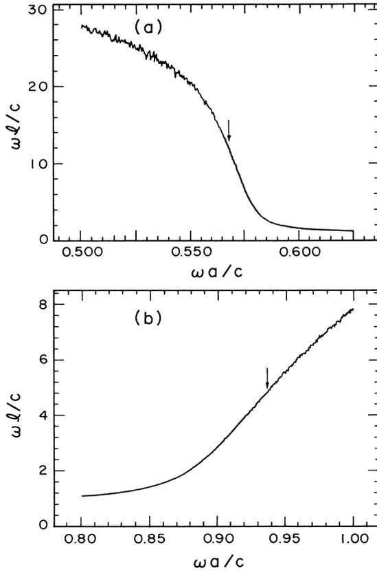
FIG. 4. Plot of  $(\omega l/c)$  (localization length) vs  $\omega a/c$  for a system with random slab widths. The results are shown for (a)  $\omega$  near the lower band-gap edge and (b)  $\omega$  near the upper band-gap edge. The curves in the figures were computed for an average over 500 random samples.
