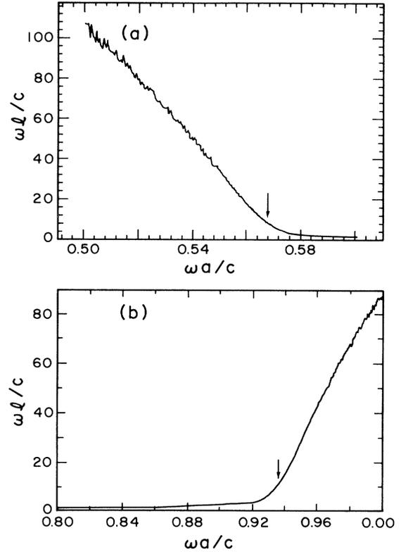
FIG. 3. Plot of  $(\omega/c)$  (localization length) vs  $\omega a/c$  for a system with random dielectric constants. The results are shown for (a)  $\omega$  near the lower band-gap edge and (b) near the upper band-gap edge. The edges of the band gaps are indicated by arrows. The curves in the figures were computed for an average over 500 random samples.
