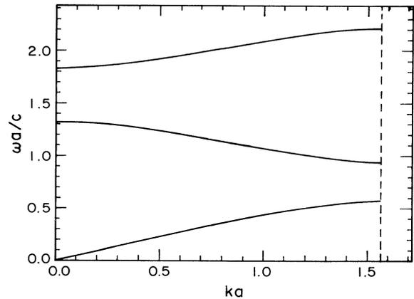
FIG. 2. The three lowest-frequency branches of the dispersion curve for electromagnetic waves propagating through the average periodic dielectric structure studied in this paper.
