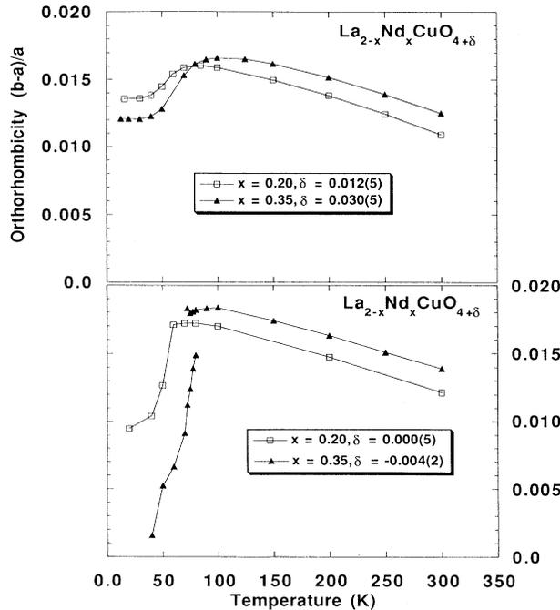
FIG. 1. Synchrotron x-ray powder diffraction measurements of orthorhombicity vs temperature for  $\text{La}_{2-x}\text{Nd}_x\text{CuO}_{4+\delta}$  prepared in air (top) and after oxygen reduction (bottom). Note that the second-order (continuous) LTO1→LTO2 transformations in oxygen excess materials become nearly or completely first order (discontinuous) in the reduced materials.
