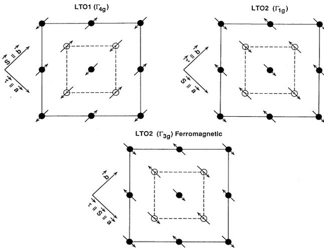
FIG. 3. Magnetic structures observed in  $\text{La}_{1.80}\text{Nd}_{0.20}\text{CuO}_{4.999(5)}$  at 80 K (LTO1,  $\Gamma_{4g}$ ), 8 K (LTO2,  $\Gamma_{1g}$ ), and  $T < 6$  K (LTO2,  $\Gamma_{3g}$ , ferromagnetic). The perspective is looking down the  $c$  axis, and the solid and open circles represent  $\text{Cu}^{2+}$  ions in adjacent layers. The directions of the  $\text{Cu}^{2+}$  moments ( $\mathbf{S}$ ) and the antiferromagnetic propagation vectors ( $\boldsymbol{\tau}$ ) are also shown.
