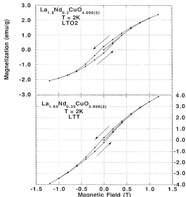
FIG. 4. Magnetic hysteresis curves at 2 K for (top)  $\text{La}_{1.8}\text{Nd}_{0.2}\text{CuO}_{4.000(5)}$  and (bottom)  $\text{La}_{1.65}\text{Nd}_{0.35}\text{CuO}_{3.996(2)}$ . The arrows indicate the direction in which the magnetic field was changed during data collection.
